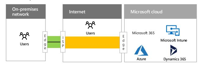
With an Internet connection, the only part of the traffic path to the Microsoft cloud that you can control (and have a relationship with the service provider) is the link between your on-premises network edge and your ISP (shown in green).
