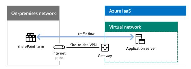
The application locates the IP address of the SharePoint farm using the on-premises DNS and all traffic goes over the site-to-site VPN connection.
