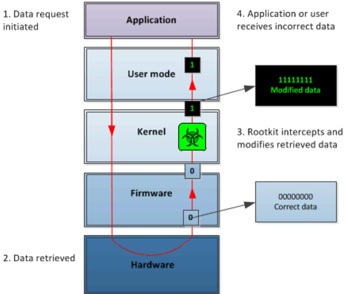
Figure 1. Possible effect of a kernel mode rootkit compromise
