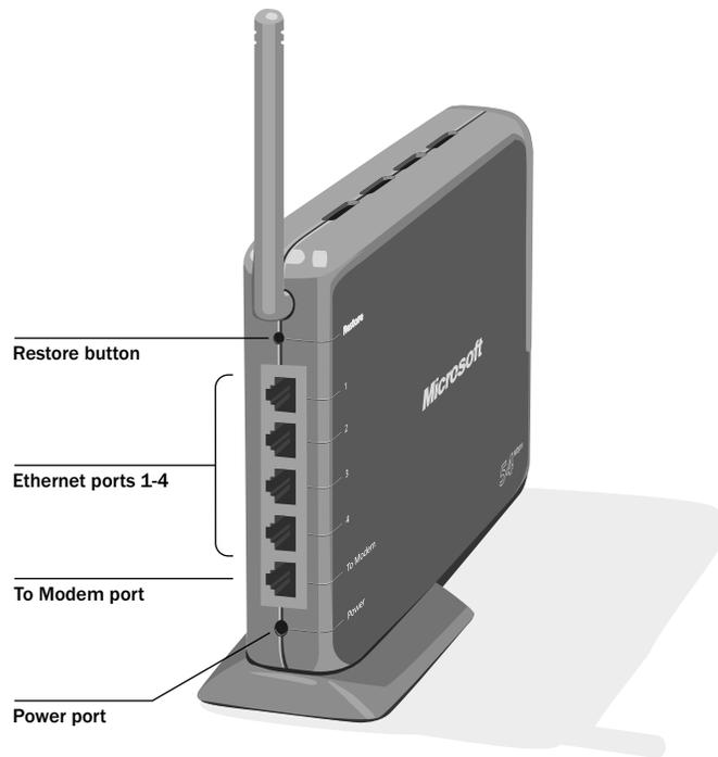
On the back of the base station, you will find a Power port, a To Modem port, four numbered Ethernet ports, and a Restore button.
