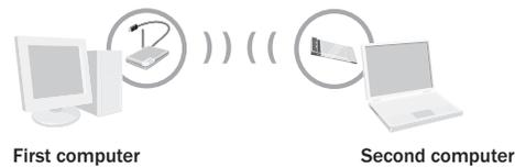
You can use the same adapter to join different networks (and different types of networks) at different times. For example, you might use your adapter to connect to an infrastructure network at home most of the time, but occasionally you might use your adapter to set up a temporary ad hoc network to share files with a colleague when you travel together on business.
