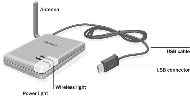
The USB adapter plugs into a computer's USB port. USB ports are rectangular and about a half-inch wide. They can be located on either the back or front of the computer.
