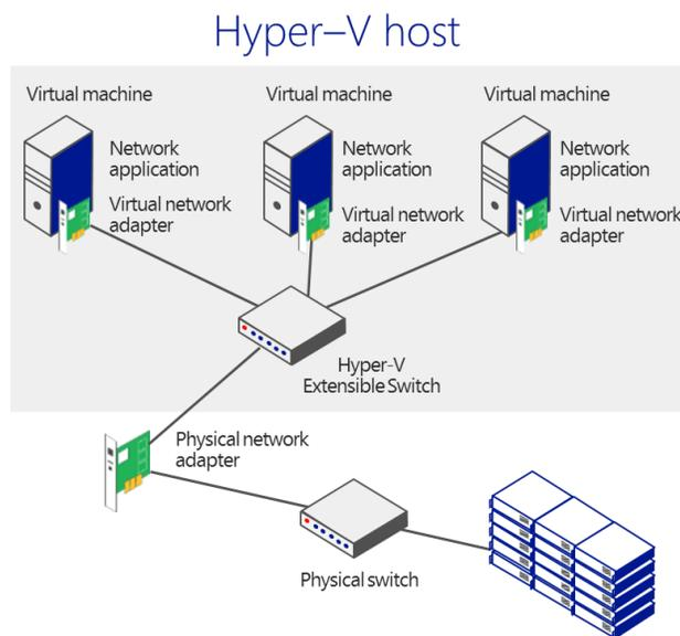
Figure 10 – Network with Hyper-V Extensible Switch
