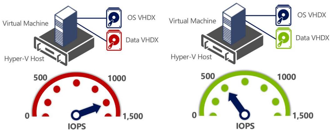
Figure 3 – Storage QoS in Action: Disabled on the left, and then enabled on the right
