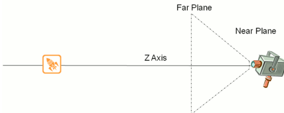
Figure 2. New camera position with incorrect view space
