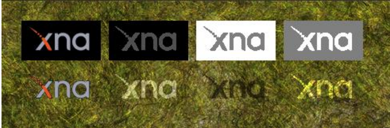
Figure 1. This picture illustrates four common blend modes. From left to right: Alpha blending, Additive blending, Multiplicative blending, and 2X Multiplicative blending. The top image in each column is the source image and below, it's effect when added to the destination.
