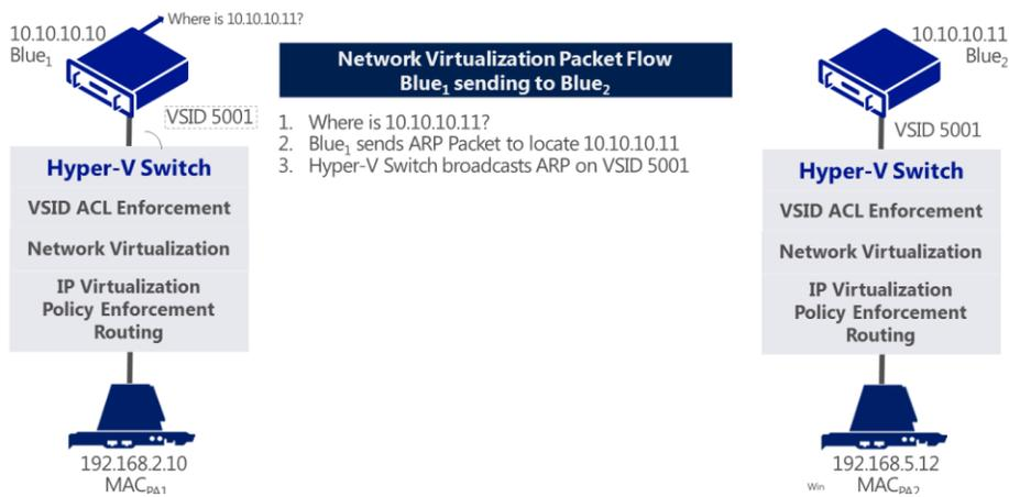
Figure 4: The Hyper-V Switch broadcasts ARP on VSID 5001.
