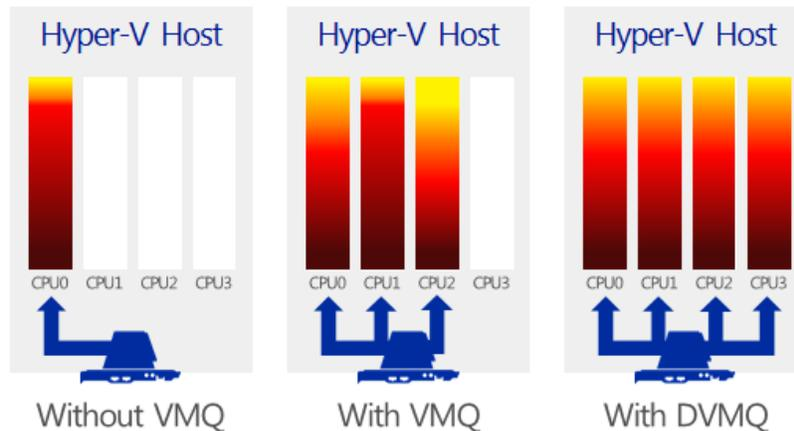
Figure 22: Different models with and without VMQ.
