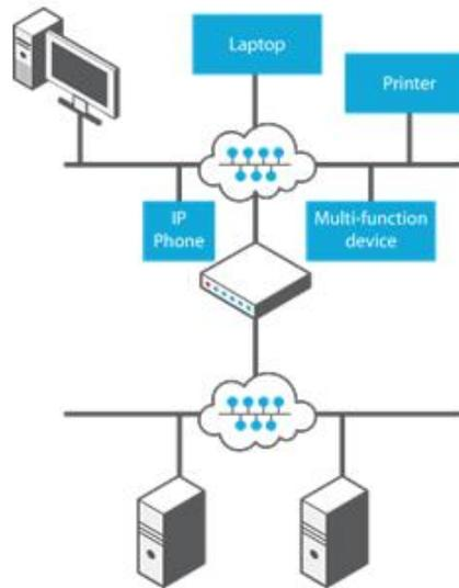
Figure 17: DHCP Server Failover in load-sharing mode.
