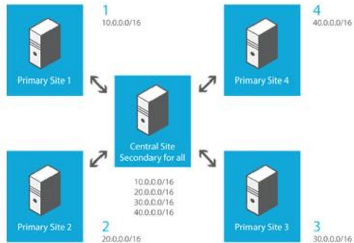
Figure 16: DHCP Server Failover in hot standby mode.
