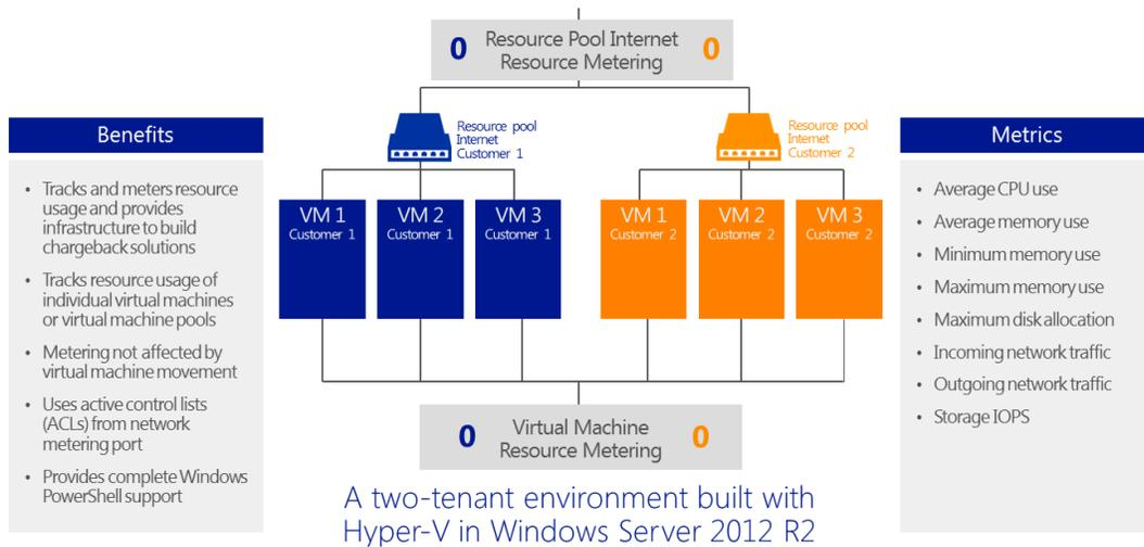
Figure 27: A multi-tenant environment built with Hyper-V.
