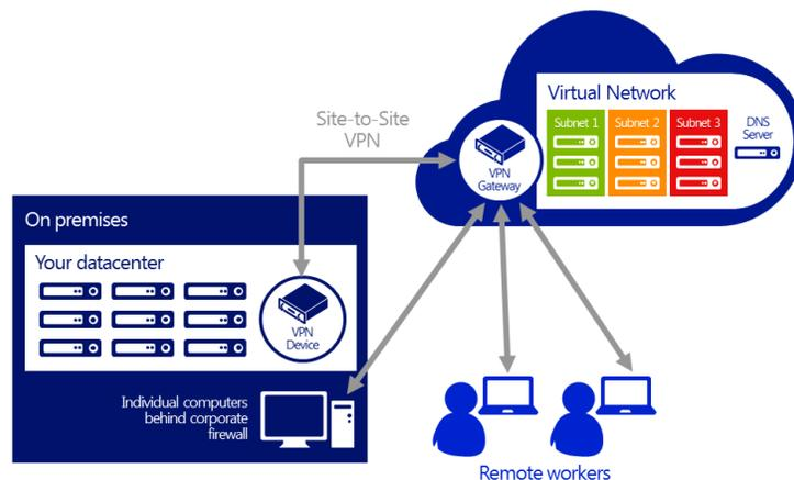
Figure 37: Virtual Network in Windows Azure set up.
