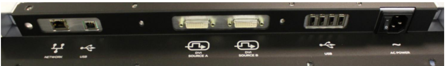
Figure 8. Connection ports from left to right: Ethernet (network), USB connection to computer, DVI (2), USB hub ports for stylus charging and accessories, and AC power
