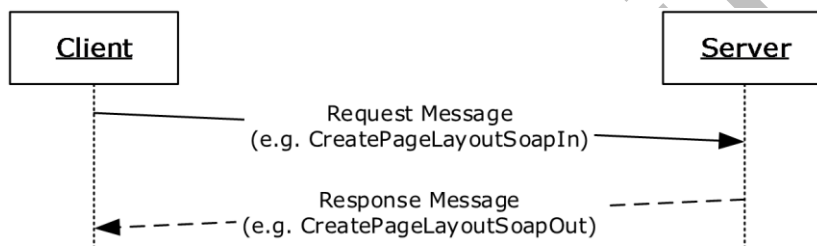
Figure 2: Sequence diagram showing the typical message pattern
