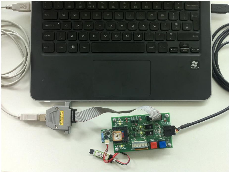
Figure 15 - Hardware connections before reprogramming the Mataki board
