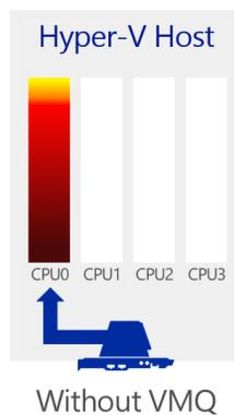
Figure 8 – Hyper-V Host Processing Network Traffic on CPU0 with no VMQ Enabled
