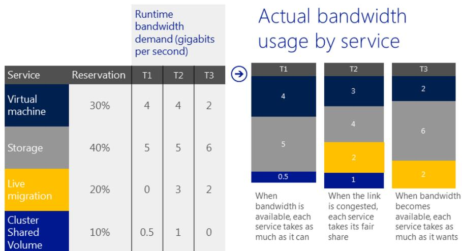
Figure 15 – Assigning minimum bandwidth to services
