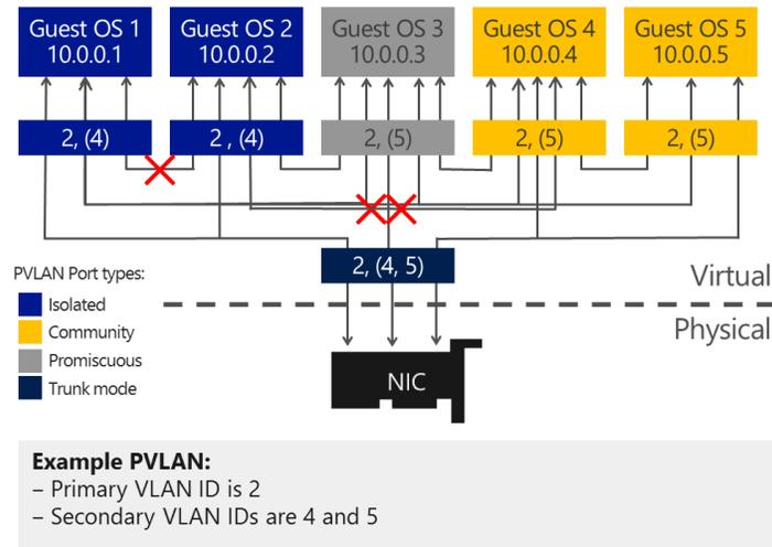
Figure 27 – Example PVLAN with primary VLAN ID 2
