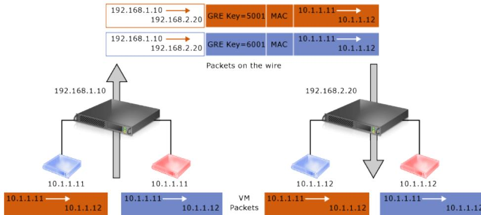
Figure 45 – Network virtualization - NVGRE encapsulation
