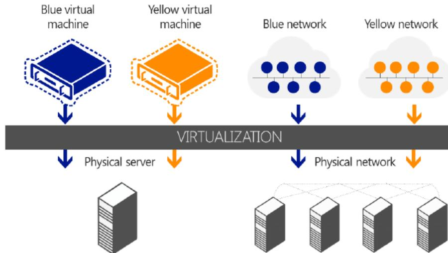
Figure 42 – Server virtualization versus network virtualization
