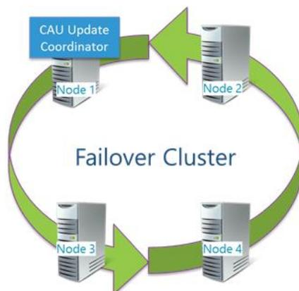
Figure 59 – The CAU Update Coordinator runs on the cluster in Self-Updating Mode.
