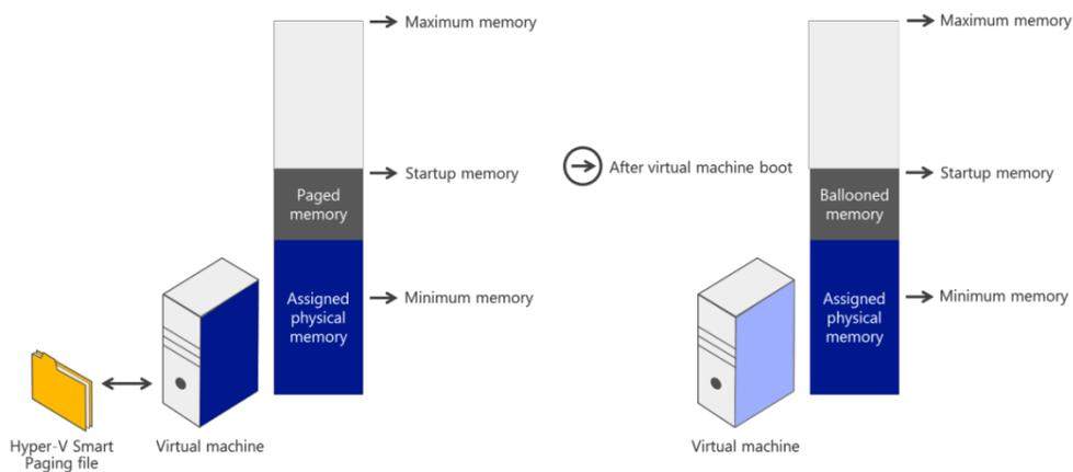
Figure 13 – Removing paged memory after virtual machine restart
