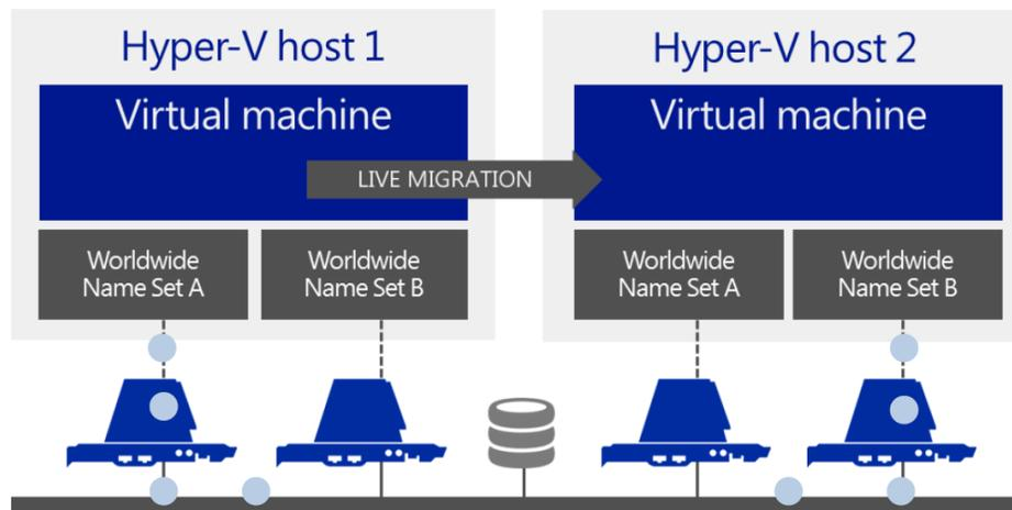
Figure 4 - Alternating WWN addresses during a live migration
