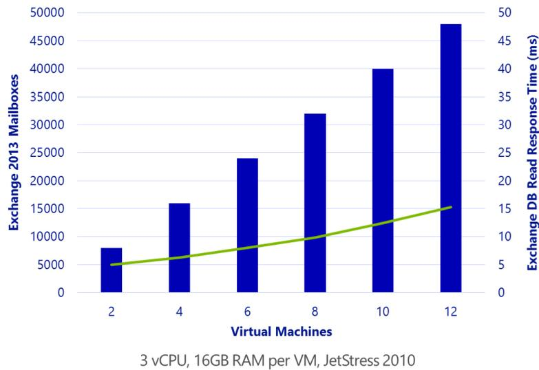
Figure 23 – Graph of virtualized Exchange 2013 scalability
