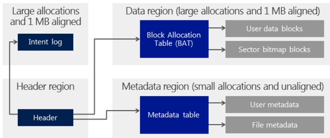
Figure 3 - The VHDX hard disk format
