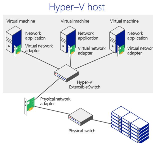
Figure 26 – Network with Hyper-V Extensible Switch
