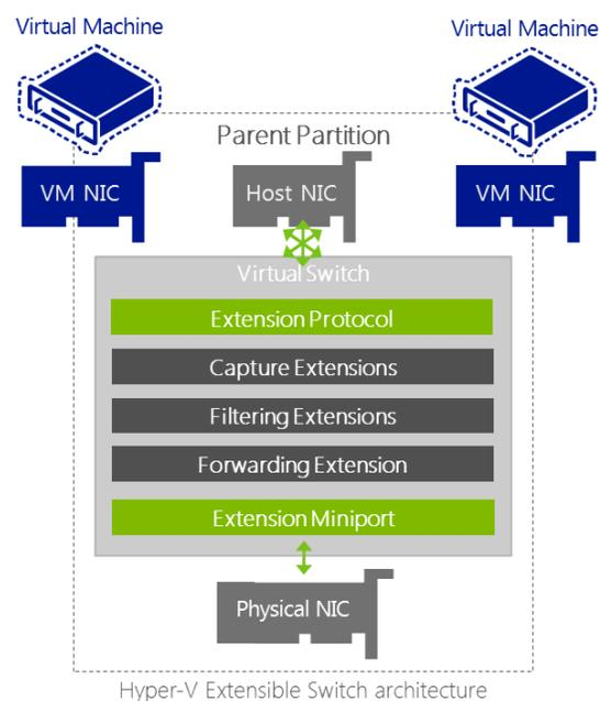
Figure 28 – Architecture of the Hyper-V Extensible Switch
