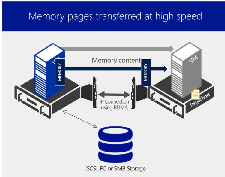
Figure 34 – Live Migration with SMB using RDMA-enabled NICs
