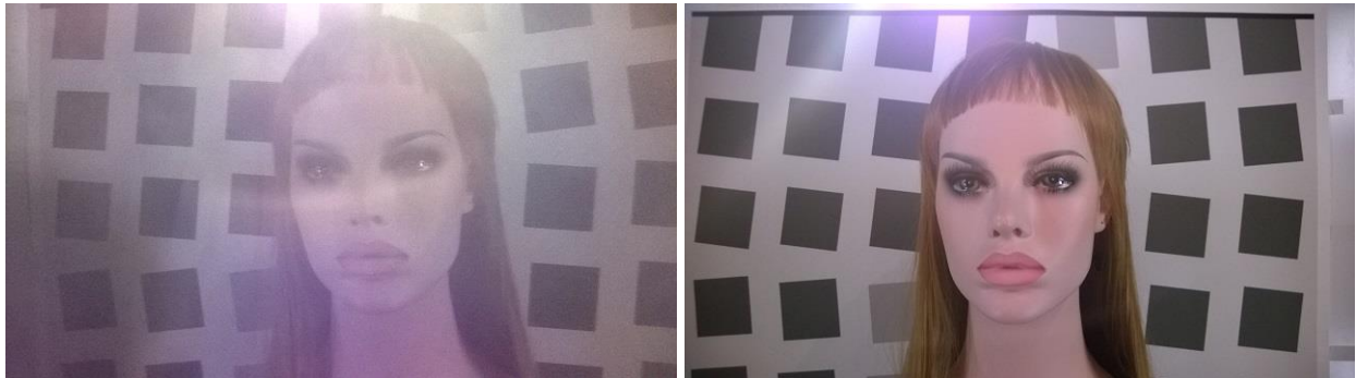
Figure 19: Image of a scene with overhead lighting from the front camera (left) and rear camera (right) of a mobile phone. The cover glass of the rear camera has anti-reflective coating, which improves the veiling glare; good lens hood can have the similar improvement
