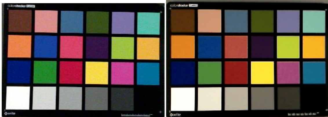
Figure 14: Left: SNR=30.6 dB; Right: SNR=41.9 dB
