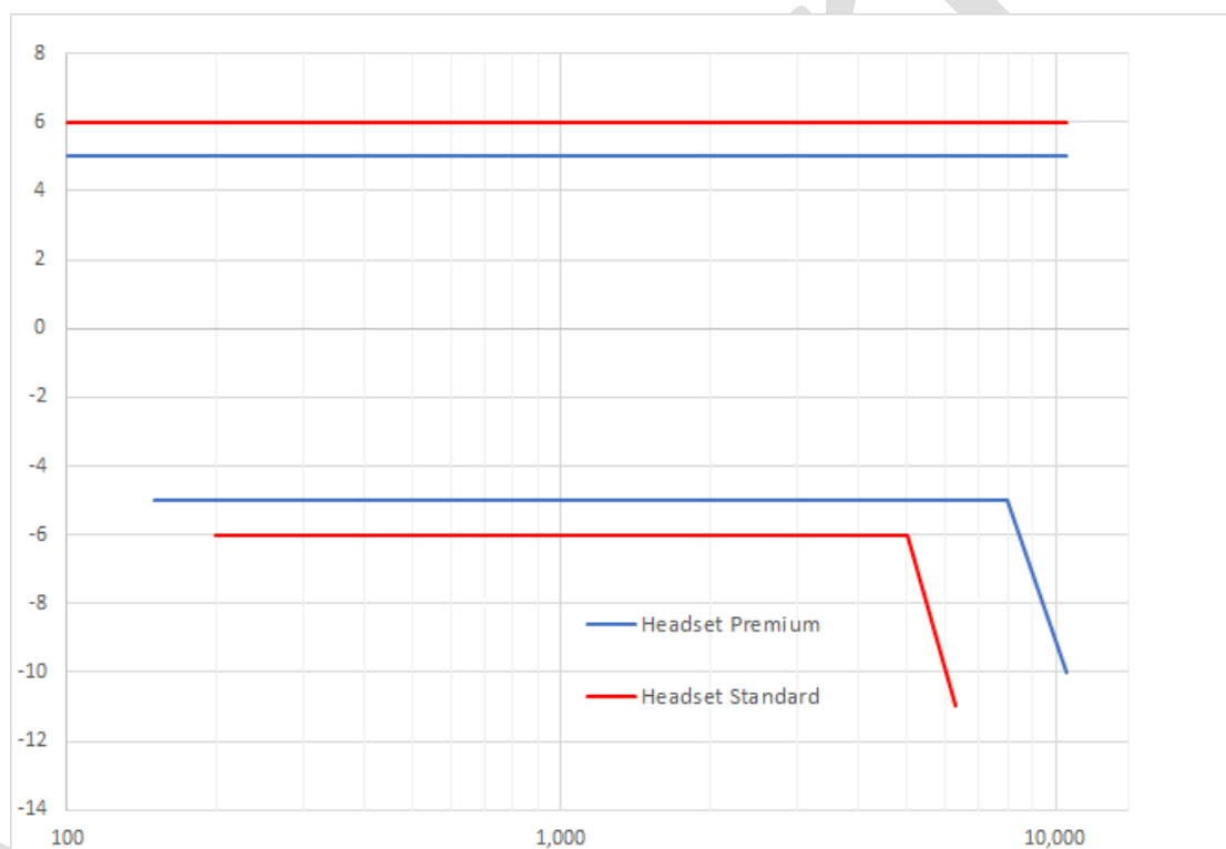
Figure 5: Headset send frequency response mask
