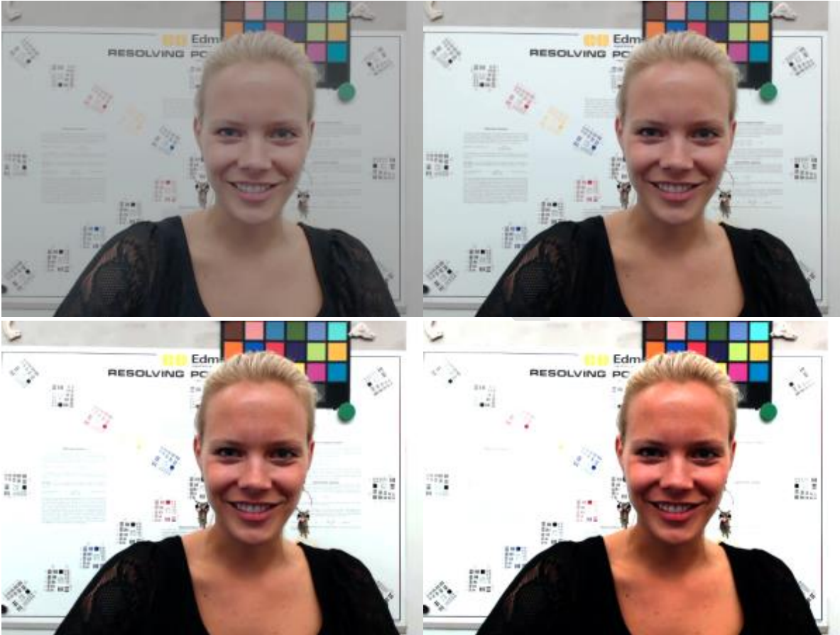
Figure 13: Upper-Left: gamma=0.3, Upper-Right: gamma=0.5, Bottom-Left: gamma=0.7, Bottom-Right: gamma=0.9
