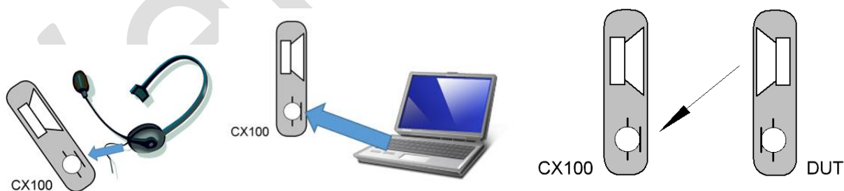
Figure 4: Audio path for measuring DUT receive latency
