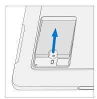
7. **Install rSSD 3IP screw in both devices** – Use a 3IP screwdriver to install the rSSD screw until it is just snug and seated, and then turn another 45 degrees (1/8 turn) or until screw is fully fastened.
