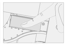
5. **Apply TDM to Bucket** – Hover the TDM and remove the PSA Liners to expose adhesive. Align the TDM along the bottom edge first (Toe-in) and lower after alignment is found. Ensure that the glass sits flush in the IBC and does not rest anywhere on top of the IBC lip.
