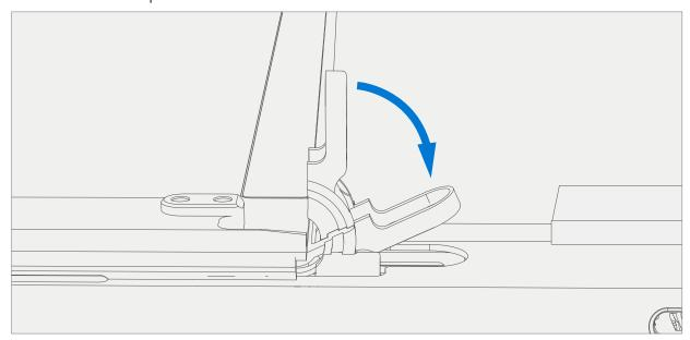
6. **Remove Kickstand** – Using the palm of your hand, firmly hold the device down from the center of the IBC. Simultaneously, grip the kickstand off-center between your thumb and index finger and firmly pull. Pull with a moderate amount of force until the foam inserts slide out of the device. If the kickstand is stuck, ensure it is not caught on the hinges.
