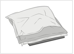
Shift second 9 kg steel shot bag to top edge of the device Bond for 3 minutes
