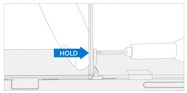
4. **Lay Kickstand Down** – Lay the kickstand flat against the IBC. Be careful not to jostle the kickstand in this position as it may cause abrasions on the IBC.
