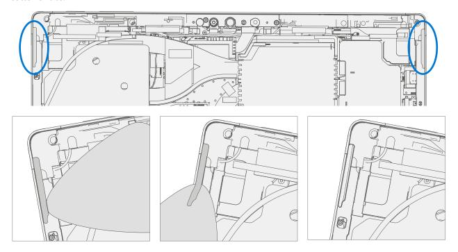
7. **Inspect for Antenna Deck (LTE Only)** – After removing the TDM on LTE devices, inspect the antenna deck gold traces. The passing criteria is shown below. Devices with damaged traces require **whole unit exchange**.
