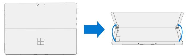
3. **Remove hinge screws** – Using the 3IP (Torx-Plus) driver, loosen all four hinge screws by 2-3 rotations. With the screws loose, use your finger to hold the back of the kickstand behind each hinge while fully removing the two hinge screws. Ensure screws do not fall into the hinge opening.
