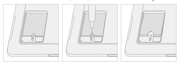
3. **Remove rSSD** – The rSSD should lift upwards to ~15 degree tilt after screw is removed. Carefully grab sides of rSSD case and pull out of main board socket at same ~15 degree angle.
