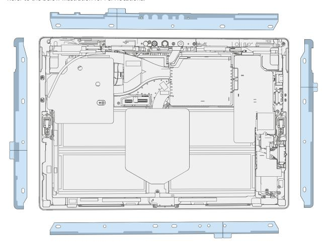
4. **Connect TDM FPCs** – While supporting the TDM with one hand, connect the TDM FPCs by pressing them into the mainboard. Install a new shield over the TDM FPCs. Ensure all edges of the shield are snapped into place.
