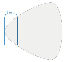
2. **Debonding TDM** – Place the device face up on a Soft ESD safe mat. Replace the iFixit pick if all the tips look scratched or deformed. Securing the device with one hand insert one of the iFixit pick tips into the right speaker area. Carefully cut the PSA applying a steady force along all edges of the TDM. Limit the pick depth to 8 mm. Run the pick 2 times around all edges of the TDM.
