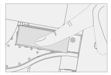
5. **Apply TDM to Bucket** – Hover the TDM and remove the PSA Liners to expose adhesive. Align the TDM along the bottom edge first (Toe-in) and lower after alignment is found. Ensure that the glass sits flush in the IBC and does not rest anywhere on top of the IBC lip. Lightly press on the edges of the TDM to create an initial bond.
