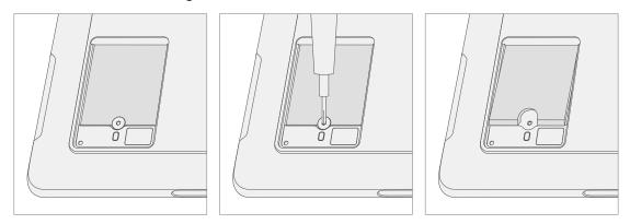
5. **Remove rSSD from both devices** – The rSSD should lift upwards to ~15-degree tilt after screw is removed. Carefully grab sides of rSSD case and pull out of main board socket at same ~15-degree angle.
