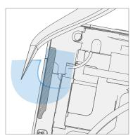
3. **TDM PSA Application** – Thoroughly clean the IBC along the TDM PSA bonding surface using IPA and a cotton swab. Wait at least 30 seconds before applying new PSA. Apply the 4 strips of PSA to the IBC. Align the PSA following the outline on the IBC. Leave the blue liner on the PSA, it will be removed at a later step. Refer to the below illustration for PSA locations.
