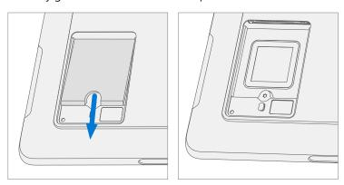
6. **Insert rSSD** – Insert the connector end of the rSSD into the rSSD connector on Main board at ~15-degree angle. Place the rSSD removed from the new device into the customer's original device. Place the customer's original rSSD into the new device.
