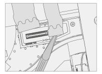
5. **Remove Residual IBC PSA** – Using flat side of a spudger, IPA, and cotton swabs, clean residual PSA off the IBC. Use only IPA and cotton swabs to clean the top edge. Ensure area around the Camera and IR Sensor is clean and free of any dust or other contamination. Wipe the area around the camera with a lint free cloth.
