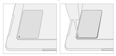
2. **Remove rSSD 3IP Screw** – Use a 3IP (Torx-Plus) driver to remove the screw securing the rSSD.
