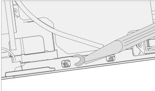
6. **Speaker Mesh** – Inspect speaker mesh for any signs of damage. Remove damaged speaker mesh from the IBC. Insert a pick between the Speaker mesh and the enclosure. Remove any residual adhesive using IPA and cotton swabs.
