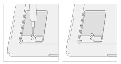
8. Install SIM (if present from the customer's old device in the new device).
