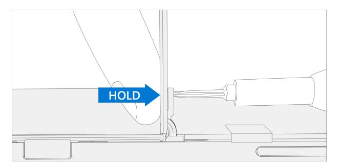
5. **Final inspection Kickstand installation** – Fold the kickstand down and peel off protective plastic from the kickstand and logo if present. Verify the side edges of the kickstand are aligned with the midframe walls and that there are no obvious steps/gaps between the kickstand and the IBC. Wipe the device thoroughly (including under the kickstand) with the microfiber cloth to remove all fingerprints.
