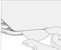
4. **Disconnect TDM FPCs** – While supporting the TDM with one hand, remove the shield lid on the TDM FPC by inserting pointed end of a spudger underneath the inner edge the of the shield. Then gently pull upwards and the shield will come off. Disconnect the TDM FPCs using the pointed end of a spudger. Do not pull on the FPCs to disconnect.
