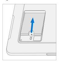
2. **Install new rSSD 3IP screw** – Use a 3IP screwdriver to install a new rSSD screw until the screw is just snug and seated, and then turned another 45 degrees (1/8 turn) or until screw is fully fastened.
