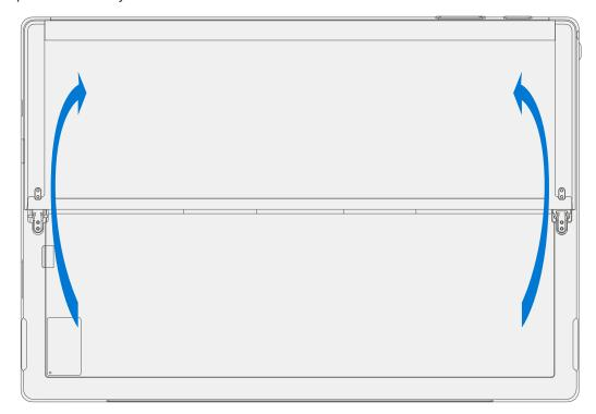
3. **Angle hinges Up** – Using your thumb or index finger, push both hinges up from 30 degrees to approximately 90 degrees. This will require a great deal of force. If necessary, place the microfiber cloth between your finger and the hinge for comfort.
