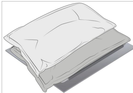
Shift second 9 kg steel shot bag to top edge of the device Bond for 3 minutes
