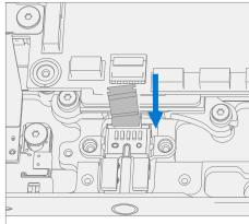
4. **Remove Audio Jack** – Remove the audio jack from the C-Cover by pulling up on the side with the FPC. Carefully move the Audio Jack from side to side during removal.
