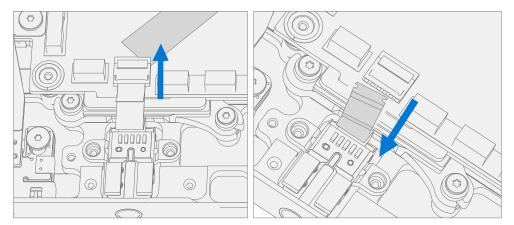
5. **Disconnect 4 Speaker Cables** – Using a plastic tool carefully release the 4 speaker connectors from the PCBA.
