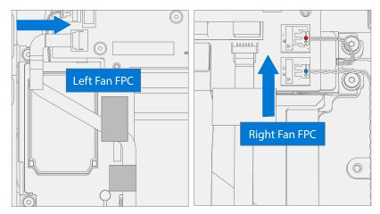
14. **Install New Fan FPC Tapes** – Refer to the picture below for tape locations. Apply 2 black tapes to the left Fan FPC securing it to the left speaker. Apply 1 black tape on the right Fan FPC securing it to the right speaker. Apply 1 black tape on the right Fan FPC securing it to the C-Cover.
