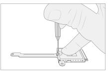
2. **Insert rSSD** - Insert the connector end of the rSSD into the receptacle on the motherboard at ~15-degree angle from horizontal.
