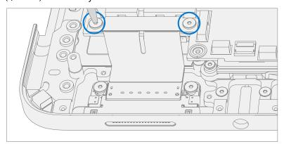
5. **Install Left I/O Bracket** – Place the left I/O bracket onto the C-Cover. Using a 3IP (Torx-Plus) driver install 3 new M1109237 screws. Turn all screws until just snug and seated, and then turn another 45 degrees (1/8 turn) or until fully fastened.
