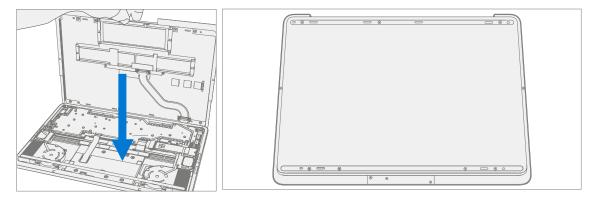
8. **New Battery Charging** – New batteries are shipped and stored at low states of charge in compliance with shipping regulations. They should be charged to at least 50%. This step will take between 20 minutes and 1 hour and is needed to validate full functionality of the new battery. Carefully place device right-side up. Open device, connect the power supply, and power it on.
