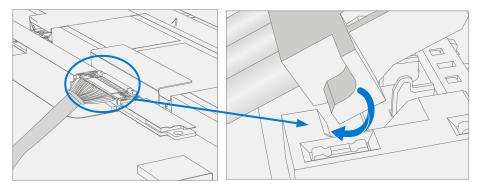
b. Press down on the tip of the connector on left and right sides. A click should be heard and felt on each side
