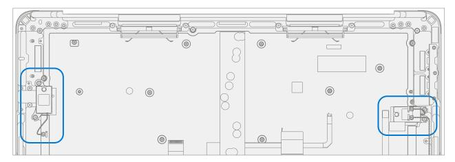
2. **Install Fans** – Install 4 foam grommets on the new C-Cover. Install the previously removed left and right fans onto the C-Cover. Using a 3IP screwdriver install 1 new M1007493 screw in each fan. Turn all screws until just snug and seated, and then turn another 45 degrees (1/8 turn) or until fully fastened.
