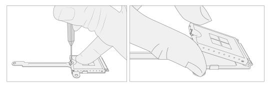
**IMPORTANT:** The 2230 rSSD bracket is reused when installing a new 2230 rSSD.
