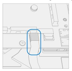
10. **Connect Keyset Backlight FPC** – Ensure the lock is released on the Keyset Backlight FPC connector. Install the Keyset Backlight FPC into the PCBA connector. Secure the connector lock.
