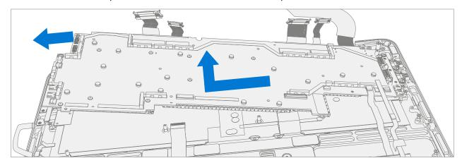
17. **Remove USB-C FPC Retainer** – Carefully set PCBA on ESD workbench with thermal module facing up. Using a 3IP (Torx-Plus) driver remove the 3 screws securing the USB-C FPC retainer to the PCBA. Remove the FPC retainer.
