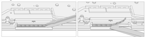
b. **Cleaning** – Remove any adhesive tape remnants from the C-Cover and clean off any glue residue with 70% or greater Isopropyl Alcohol.
