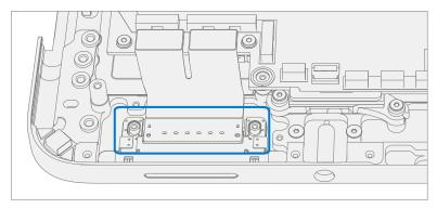
2. **Connect Surflink FPCs** – Align the FPC's connectors to the PCBA and press down.
