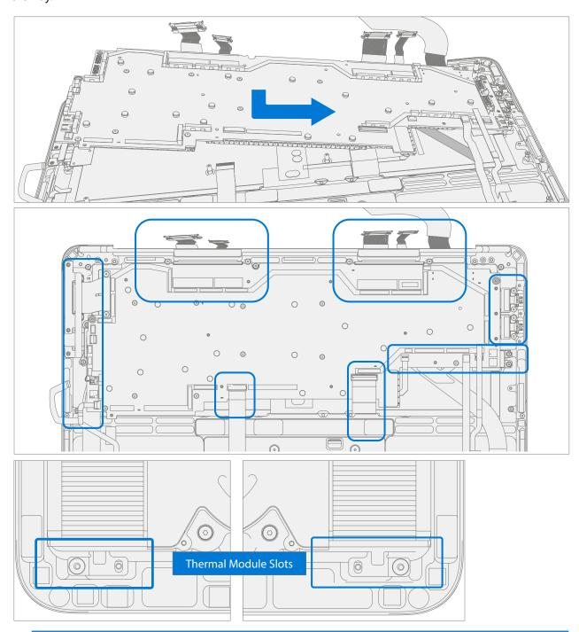
! CAUTION: Verify the 15 cables and FPC's are not captured under the PCBA. The Fan and Wireless Pen Charger FPCs route over the thermal heat pipe. Ensure the thermal module slots align over the posts in the C-Cover.
