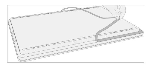
IMPORTANT: Along the front edge pull the cosmetic plate in a tight 'U' shape to prevent the black spacer from lifting up with the cosmetic plate. A replacement black spacer is included with the new Cosmetic Plate in situations where it is removed.
