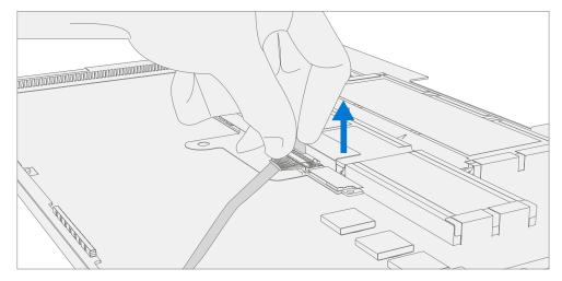
b. Using the "Pull" tab, slide the connector carefully towards the battery to release the latches and remove the cable.
