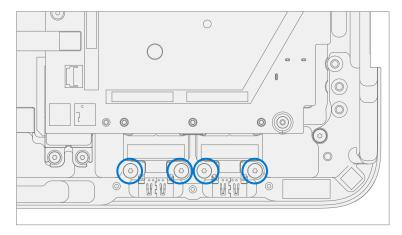
13. **Remove Fan FPC Tapes** – Carefully remove the 4 black tapes securing the fan FPCs.
