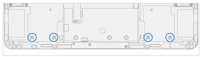
3. **Remove Tweeters** – Use 3IP screwdriver to remove the screws from the left and right tweeters. Remove the tweeters.
