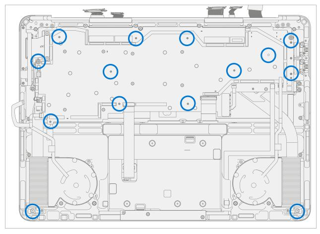
16. **Remove PCBA** – Start by holding the SL connector cable out of the way and slightly pick up the left side of the PCBA. Rotate the PCBA up and out. Ensure the USB-C connectors separate from the C-Cover.
