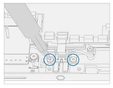
3. **Disconnect Audio Jack FPC** – Release the lock on the Audio Jack FPC connector. Remove the Audio Jack FPC from the PCBA connector.
