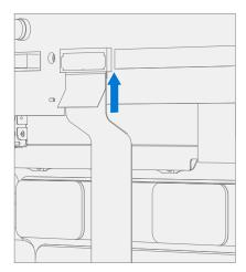
13. **Connect Fan FPCs** – Ensure the locks are released on the left and right Fan FPC connectors. Install the left and right Fan FPCs into the PCBA connectors. Secure the connector locks.
