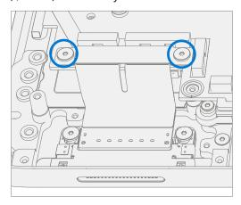
18. **Connect 4 Display Cables** – Carefully connect the 4 display cables into the PCBA connectors. Ensure the connections are fully seated and the locking buckles are engaged.
