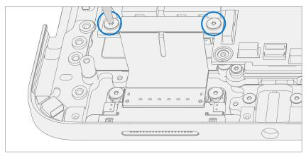
3. **Remove Surflink Port Screws** – Using a 3IP (Torx-Plus) driver remove the 2 screws securing the Surflink Port to the C-Cover.
