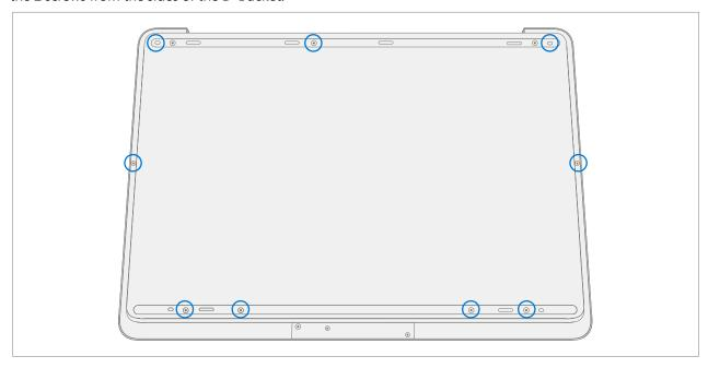
! CAUTION: All 9 screws must be removed before starting D-Bucket removal.
