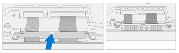
b. Ensure that the cables route over the plastic guide along the edge of the MB.
