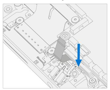
2. **Connect Audio Jack FPC** – Ensure the lock is released on the Audio Jack FPC connector. Install the Audio Jack FPC into the PCBA connector. Secure the connector lock.
