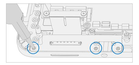
2. **Remove Surflink FPC Retainer** – Using a 3IP (Torx-Plus) driver remove the 2 screws securing the Surflink FPC retainer to the PCBA. Remove the cable retainer.
