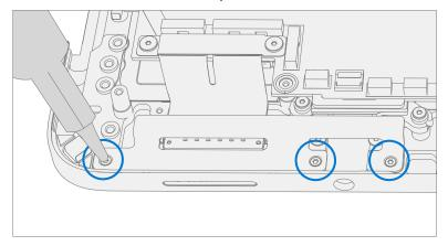
2. **Remove Audio Jack Screws** – Using a 3IP (Torx-Plus) driver remove the 2 screws securing the audio jack to the C-Cover.
