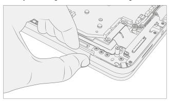
d. Verify a 0.2 mm plastic thickness gauge can slide easily in the hinge gap.
