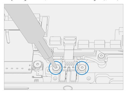
4. **Install Left I/O Bracket** – Place the left I/O bracket onto the C-Cover. Using a 3IP (Torx-Plus) driver install 3 new M1109237 screws. Turn all screws until just snug and seated, and then turn another 45 degrees (1/8 turn) or until fully fastened.
