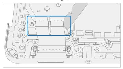
5. **Remove Surflink Port** – Remove the Surflink Port from the C-Cover.
