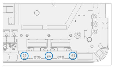
12. **Remove USB-C Screws** – Using a 3IP (Torx-Plus) driver remove the 4 screws securing the USB-C connectors to the C-Cover.
