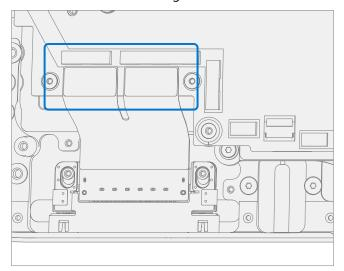
3. **Install new Surflink Port screws** – Using a 3IP (Torx-Plus) driver install 2 new M1149393 screws. Turn all screws until just snug and seated, and then turn another 45 degrees (1/8 turn) or until fully fastened.
