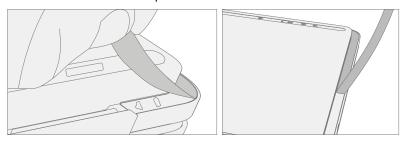
**IMPORTANT:** Pull the cosmetic plate away from the device at an angle to prevent scratching the D-Bucket.
