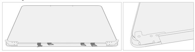
3. **Install display module onto C-Cover** – While holding the C-Cover with one hand. Carefully align the hinges into the pockets on the C-Cover. Apply a 1-inch light duty spring clamp to the left hinge.
