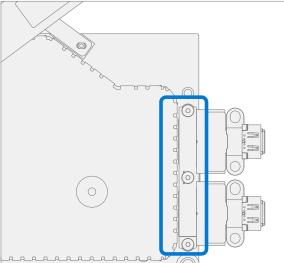
3. **Install PCBA** – Install the right side of the PCBA down and into the C-Cover. Ensure the USB-C connectors are aligned into the C-Cover. Lower the left side of the PCBA into the C-Cover while holding the Surflink FPC out of the way.
