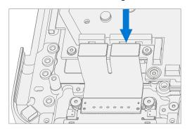
17. **Install Surflink FPC Retainer** – Place the FPC retainer over the Surflink FPCs. Using a 3IP (Torx-Plus) driver install 2 new M1149393 screws. Turn all screws until just snug and seated, and then turn another 45 degrees (1/8 turn) or until fully fastened.
