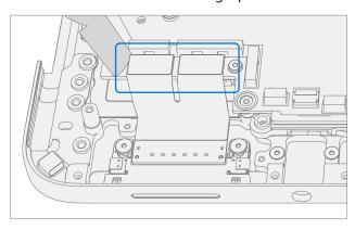
4. **Disconnect Audio Jack FPC** – Release the lock on the Audio Jack FPC connector. Remove the Audio Jack FPC from the PCBA connector.
