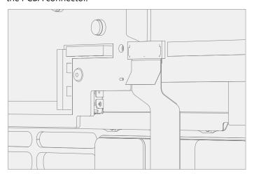
8. **Disconnect Keyset FPC** – Release the lock on the Keyset FPC connector. Remove the Keyset FPC from the PCBA connector.
