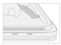
**2. Cleaning** – Remove any adhesive tape remnants from the D-Bucket and clean off any glue residue with 70% or greater Isopropyl Alcohol.
