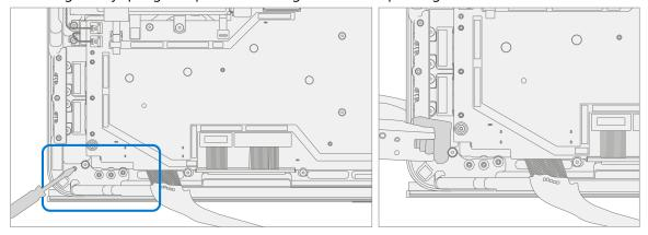
6. **Remove Right Hinge Screws** – Using a 6IP (Torx-Plus) driver remove the 4 screws on the right hinge.
