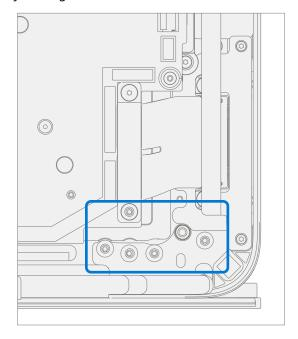
5. **Pre-fasten left hinge screws** – Remove the 1-inch light duty clamp form the left hinge. Assemble 4 new M1150078 screws in the left side hinge and tighten until just snug.
