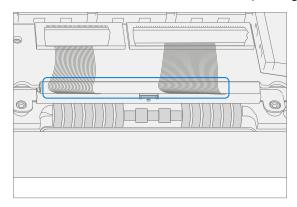
c. Using a 3IP (Torx-Plus) driver install the 2 new M1177566 screws in each cable tensioner. Turn each screw until just snug and seated, and then turn another 45 degrees (1/8 turn) or until screws are fully fastened.
