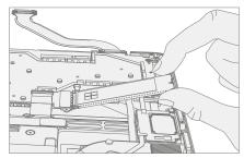
3. **Install new rSSD screws** - Using a 3IP (Torx-Plus) driver install 2 new M1167371 rSSD screws. Turn all screws until just snug and seated, and then turn another 45 degrees (1/8 turn) or until fully fastened.
