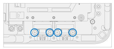
8. **Install Right I/O Bracket** – Place the Right I/O bracket onto the C-Cover. Using a 3IP (Torx-Plus) driver install 3 new M1109237 screws. Turn all screws until just snug and seated, and then turn another 45 degrees (1/8 turn) or until fully fastened.
