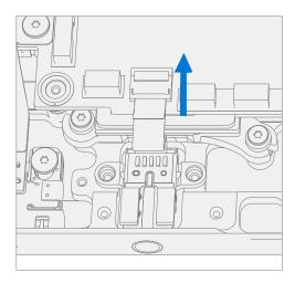
16. **Connect Surflink FPCs** – Align the FPC's connectors to the PCBA and press down.
