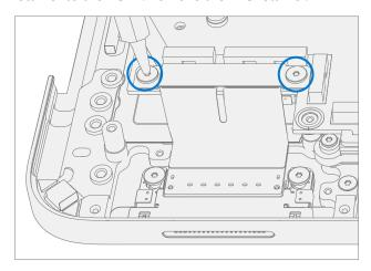
3. **Disconnect Surflink FPCs** – Using a plastic tool disconnect the Surflink FPCs from the PCBA.
