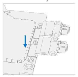
2. **Install USB-C FPC Retainer** – Place the FPC retainer over the USB-C FPCs. Using a 3IP (Torx-Plus) driver install 3 new M1167780 screws securing the Surflink FPC retainer to the PCBA. Turn all screws until just snug and seated, and then turn another 45 degrees (1/8 turn) or until fully fastened.
