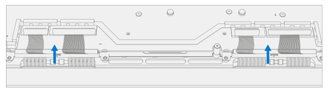
a. Ensure that the cables route over the plastic guide along the edge of the MB
