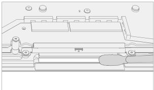
c. **Install New Display Cable Foam** – Remove the liner from the display cable foam. Align the display cable foam adhesive side down onto the C-Cover over the silver surface. Press down on the foam for 30 seconds. Repeat this for each side of the C-Cover.
