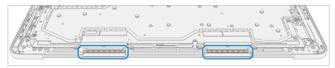
a. **Remove left and right foam** – Using a plastic tool remove the display cable foam from the left and right sides of the C-cover.
