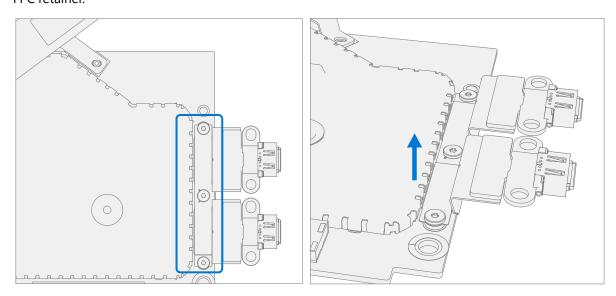
18. **Disconnect USB-C FPCs** – Using a plastic tool disconnect each USB-C FPC from the PCBA.
