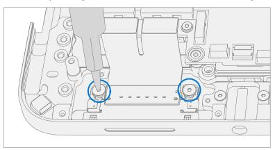
4. **Install Surflink FPC Retainer** – Place the FPC retainer over the Surflink FPCs. Using a 3IP (Torx-Plus) driver install 2 new M1149393 screws. Turn all screws until just snug and seated, and then turn another 45 degrees (1/8 turn) or until fully fastened.
