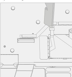
10. **Disconnect Wireless Pen Charger FPC** – Using a plastic tool carefully release the Wireless Pen Charger from the PCBA connector.
