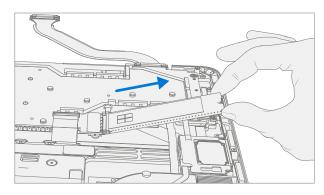
2. **Remove 2230 rSSD from bracket** – Using a 3IP (Torx-Plus) driver remove the screw securing the 2230 rSSD to the bracket and then remove the rSSD.
