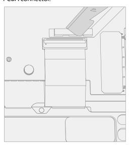
9. **Disconnect Keyset Backlight FPC** – Release the lock on the Keyset Backlight FPC connector. Remove the Keyset Backlight FPC from the PCBA connector.
