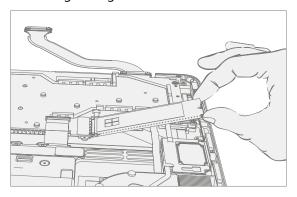
6. **Install new rSSD screws** – Using a 3IP (Torx-Plus) driver install 2 new M1167371 rSSD screws. Turn all screws until just snug and seated, and then turn another 45 degrees (1/8 turn) or until fully fastened.
