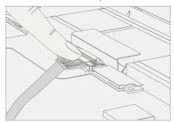
5. **Install rSSD** – Insert the connector end of the rSSD into the rSSD connector on the motherboard at ~15-degree angle.
