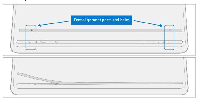
3. **Securing New Feet** - Place a ruler over one of the feet. Press down on the ruler with several fingers spaced along the length of the ruler for about 30 seconds to secure the foot. Repeat the same steps for the remaining foot.
