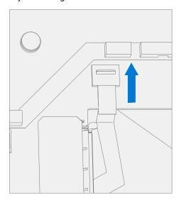
11. **Connect Keyset FPC** – Ensure the lock is released on the Keyset FPC connector. Install the Keyset FPC into the PCBA connector. Secure the connector lock.
