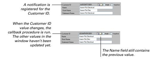
You can prevent this problem by registering separate notifications for the Customer ID and Name controls. When each value changes, the callback procedure for that control can then retrieve the correct value.
