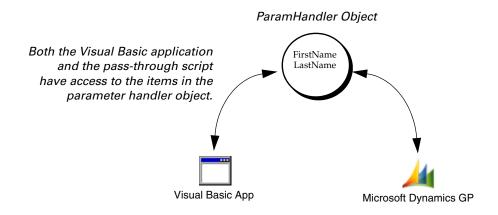
When you've created the parameter handler object, you must use the <u>SetParamHandler method</u> of the Microsoft Dynamics GP application object to specify which object in the Visual Basic application is being used as the parameter handler. This allows the pass-through sanScript to know which object to use when it sets or retrieves parameter values.
