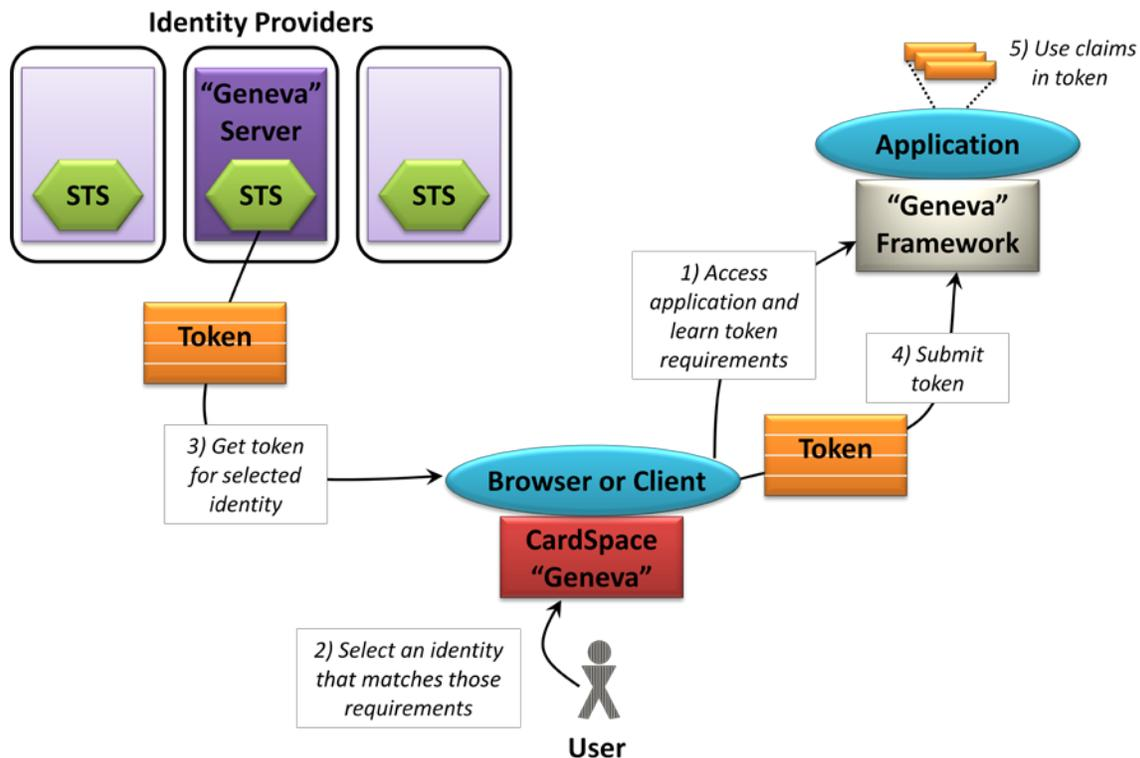
**Figure 5: The “Geneva” Server implements a Windows-based STS, CardSpace “Geneva” provides an identity selector for Windows clients, and the “Geneva” Framework is a standard library for creating claims-aware Windows applications.**
