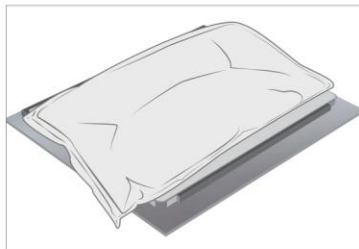
Place 9 kg steel shot bag onto device
