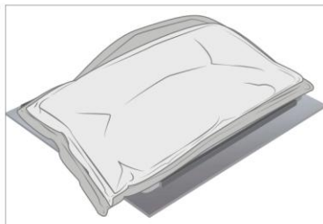
Place second 9 kg steel shot bag onto 14kg bag Bond for 5 minutes
