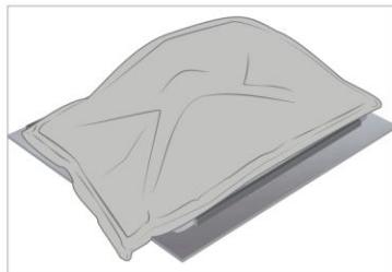
Place 14 kg steel shot bag onto device Bond for 1 minute
