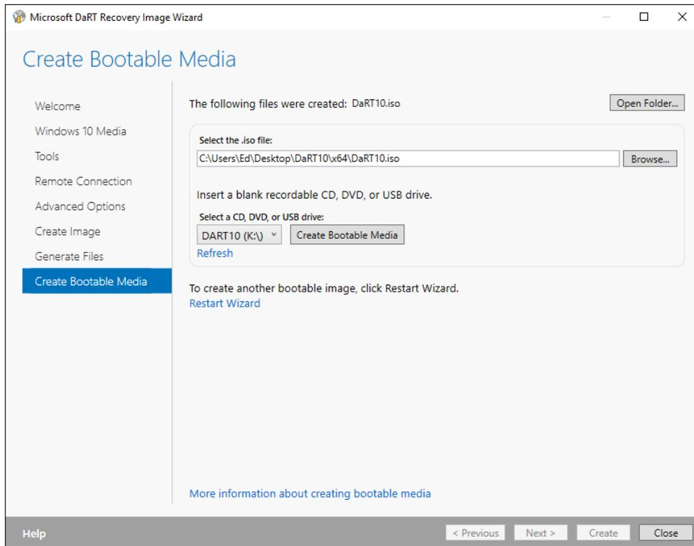
**Figure 8-15:** Immediately after creating the ISO recovery image, copy it to bootable media, label the drive, and then save it with other troubleshooting tools.
