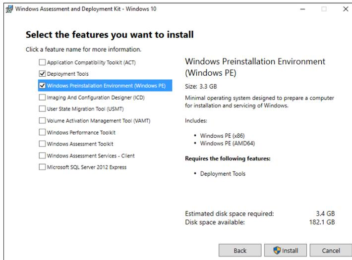
**Figure 8-8:** To create a DaRT recovery image, you must first install the Windows Assessment and Deployment Toolkit with these options selected.
