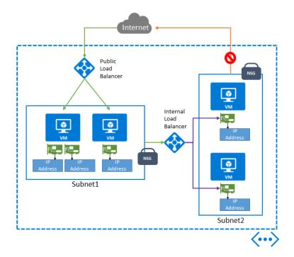
Figure 3-3 Use of both an external and an internal load balancer.
