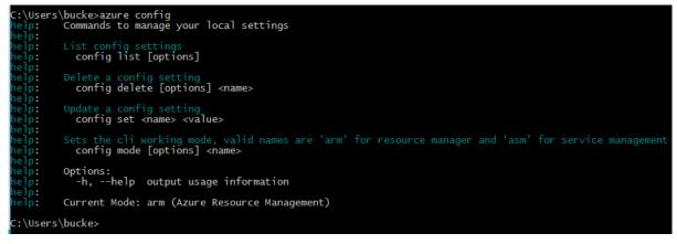
Figure 8-20 The Azure CLI configuration commands.
