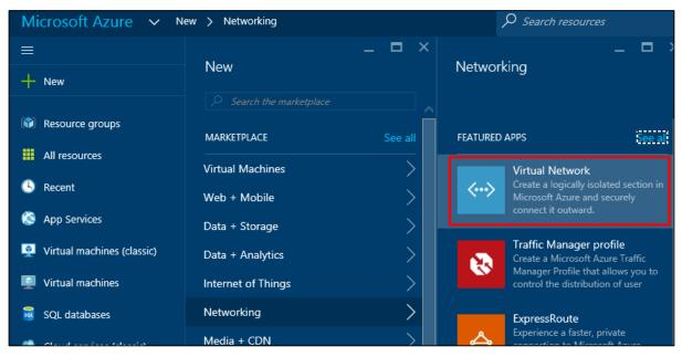
Figure 5-1 Use the Azure portal menu to create a new virtual network.
