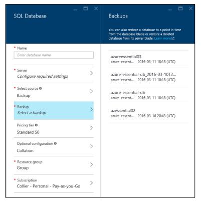
Figure 6-11 Select the desired backup as the source for a new SQL Database.
