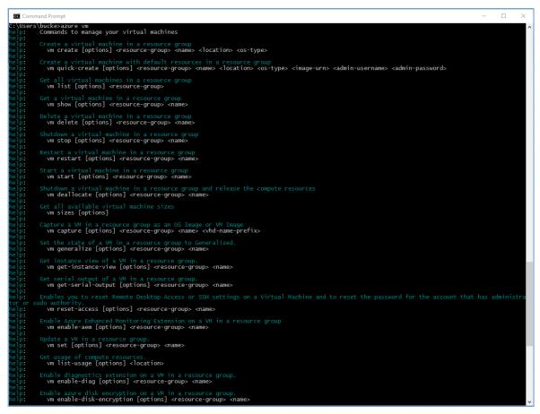
Figure 8-21 Options for working with Azure Virtual Machines in Azure Resource Manager mode.
