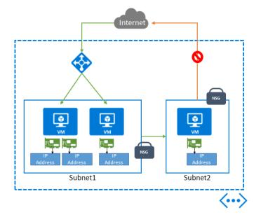
Figure 3-2 VMs in the Resource Manager model have explicit control over related network components.
