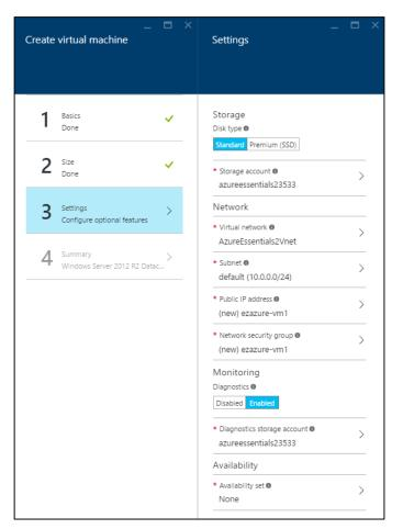
Figure 3-6 Optional configuration settings for a new Azure VM.
