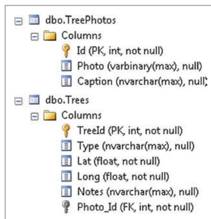
Figure 4 Using Code First Convention, Tree Gets a Non-Nullable Foreign Key to TreePhotos
