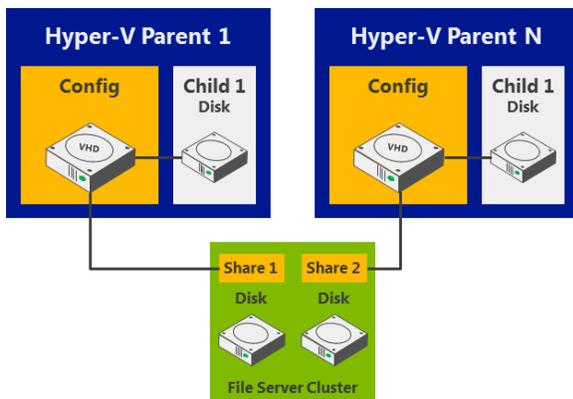
**Dual-Node File Server:** In a Dual-Node File Server, file servers can be clustered storage spaces, where shares are used for VHD storage (Figure 14). This configuration provides flexibility for shared storage, fault-tolerant storage, and low costs for acquisition and operation. It also offers continuous availability but with limited scalability.
