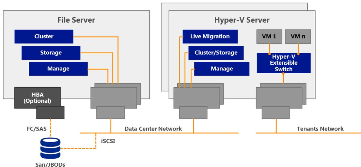
Windows QoS policies on the parent Hyper-V partition enable guaranteed levels of bandwidth to all incoming infrastructure traffic. DCB enables QoS offload capabilities to both the 10 GbE network adapter and the 10 GbE-capable switch. The tenant traffic from different tenants receives guaranteed levels of bandwidth using Hyper-V virtual switch QoS policies.
