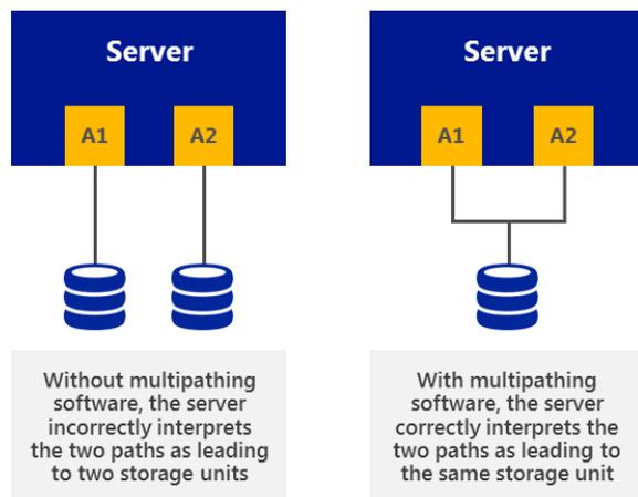
With MPIO, Windows Server 2012 efficiently manages 32 paths between storage devices and the Windows host operating system, and provides fault-tolerant connectivity to storage. Further, as more and more data is consolidated on SANs, the potential loss of access to storage resources is unacceptable. To mitigate this risk, high availability solutions like MPIO have become a requirement.
