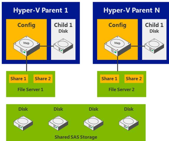
**Multi-Node File Server:** A Multi-Node File Server uses clustered Hyper-V file servers and storage spaces, where shares are used for VHD storage (Figure 15). This configuration provides flexibility for shared storage, fault-tolerant storage, and low costs for acquisition and operation. It also provides continuous availability, and Hyper-V virtual machines are highly available.
