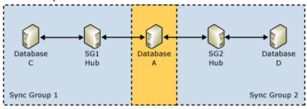
Figure 1: Two sync groups sharing a database. No synchronization loop
