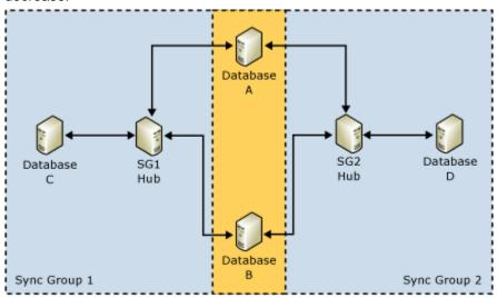
Figure 2: Two sync groups with a synchronization loop
