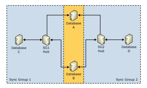
Figure 4: Use synchronization direction to prevent loops
