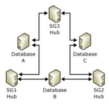
Figure 3: Three sync groups with a synchronization loop
