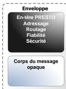
Figure 6 – Services techniques via l'enveloppe technique PRESTO.
