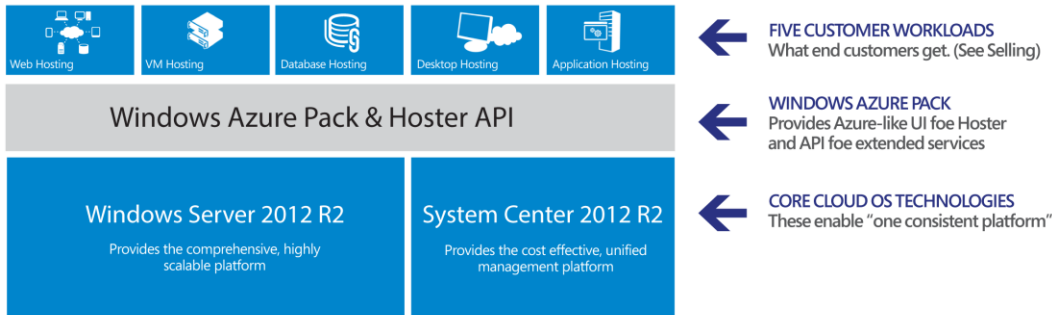
Fig. 2. Cloud OS high-level architecture, including enabled customer workloads.
