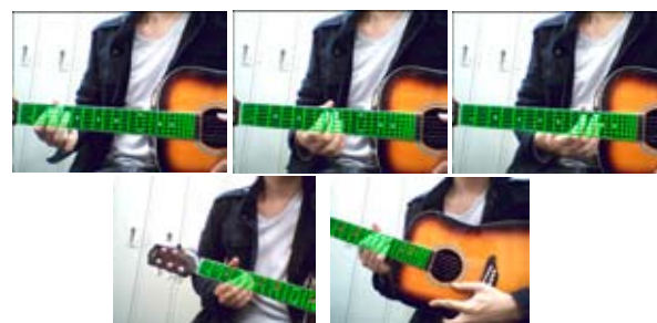
Fig. 1 Markerless guitar tracking has been achieved even when the guitar is occluded by player's hand.
