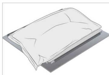
Place 9 kg steel shot bag onto device
