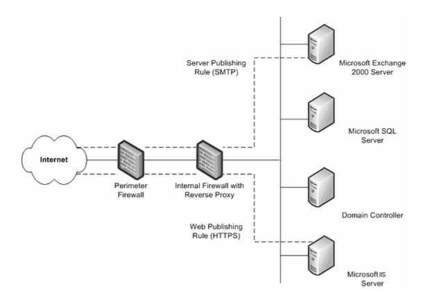
This scenario is similar to the preceding scenario after the second firewall is added. The only difference is that the internal firewall that supports reverse proxy is not an ISA Server. In this scenario, you should work closely with the managers of each firewall to define server publishing rules that adhere to the security policy.
