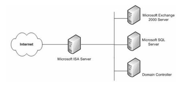
This single firewall solution is more secure than an entry-level firewall appliance and provides Windows-specific security services.
