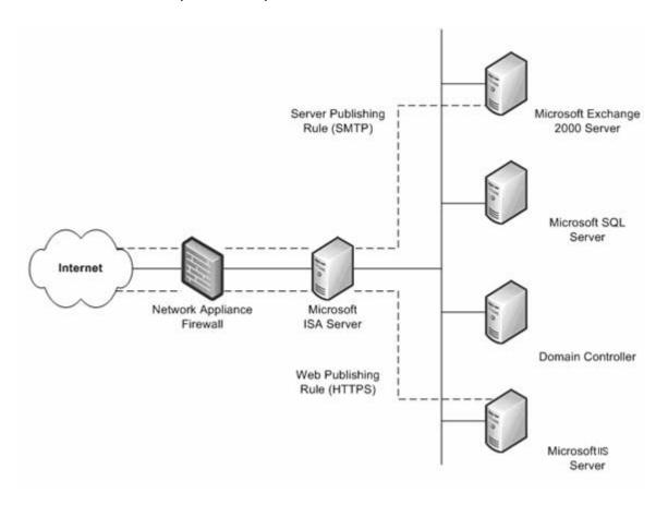
**Two Existing Firewalls** The fourth scenario involves the two firewalls implemented with an established perimeter network (DMZ). One or more of these servers provides reverse proxy services so that Internet clients are not accessing servers on the intranet directly. Instead, one of the firewalls, ideally the internal firewall, is intercepting network requests for internal servers, inspecting those packets, and then forwarding them on behalf of the Internet host.
