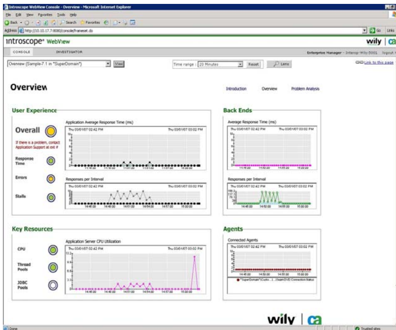
Figure 4. It is possible to launch Introscope's WebView thin client user interface from the Operations Manager console, to see more detail.
