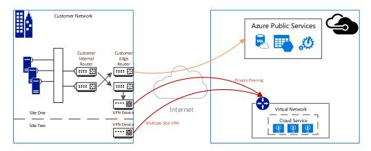
ExpressRoute connections use routers and private network paths to route traffic to Azure Virtual Network and, optionally, to the Azure public services. Private connections are made through a network provider by establishing an ExpressRoute circuit with a selected provider. The customer's router is connected to the provider's router, and the provider creates the ExpressRoute circuit to connect to the Azure Routers.
