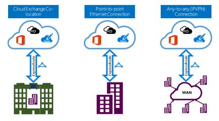
The connections between the customer's network edge and the provider's network edge are redundant as are the connections from the provider's edge to the Azure edge.
