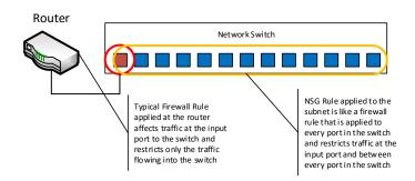
For example, if a Network Security Group is created and a Network Security Group rule is defined that denies inbound Remote Desktop Protocol (RDP) traffic for all addresses over port 3389, no virtual machine outside the subnet can connect via RDP to a virtual machine that is connected to the subnet, and no virtual machine connected to the subnet can connect via RDP to any other connected virtual machine.
