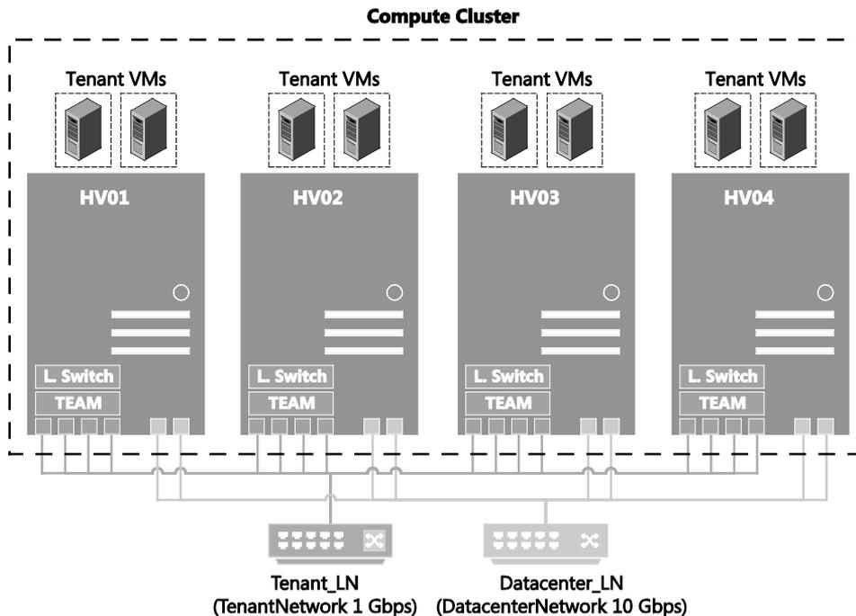
**FIGURE 1-7** Logical architecture for the compute cluster
