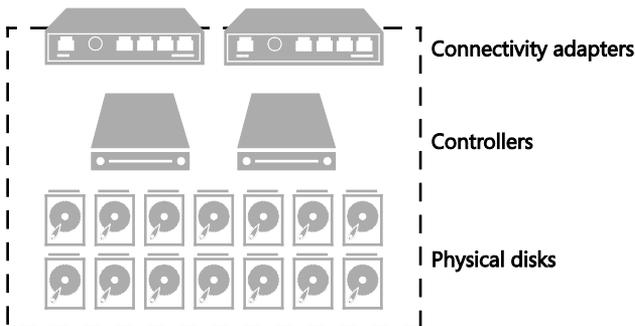
**FIGURE 1-4** Conceptual layout of SAN storage
