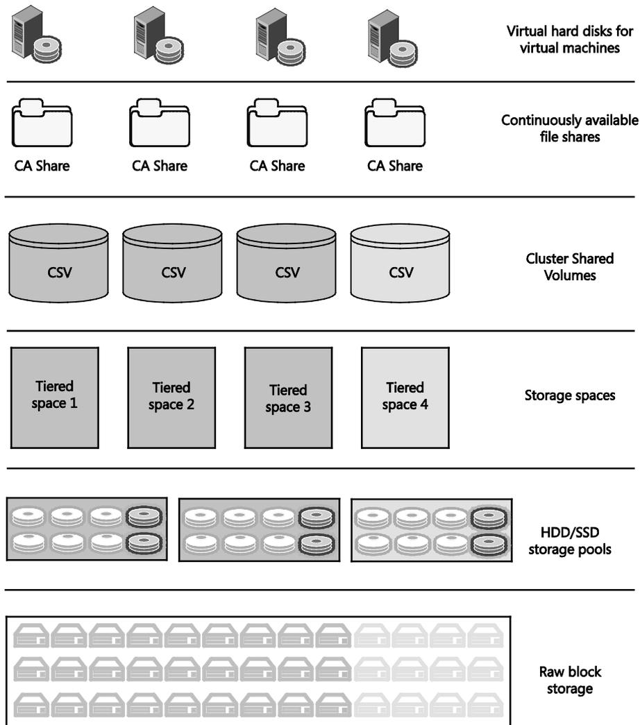
FIGURE 4-15 Layers of the Windows Server storage stack
