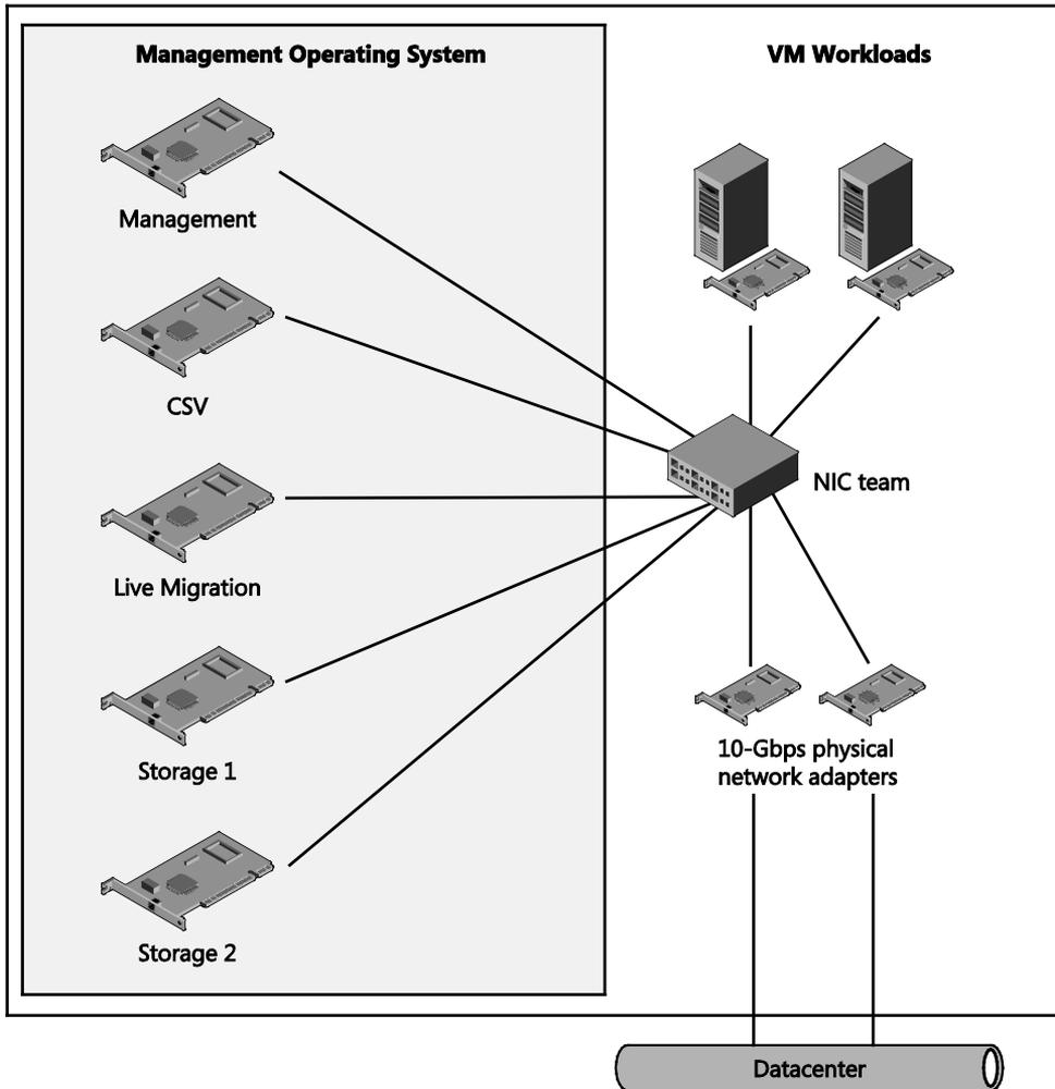
**FIGURE 5-24** Logical view of virtual network adapters
