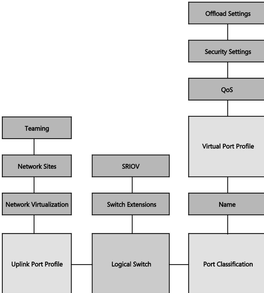
**FIGURE 3-12** Building blocks of a logical switch
