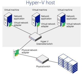
Figure 10 – Network with Hyper-V Extensible Switch
