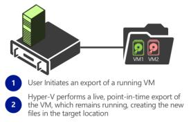
Figure 12 – Virtual Machine Live Cloning initialized and cloning the key files
