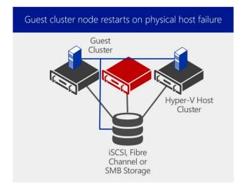
Figure 15 – A Guest Cluster running on a Hyper-V Cluster that has a single node failure
