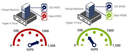
Figure 3 – Storage QoS in Action: Disabled on the left, and then enabled on the right
