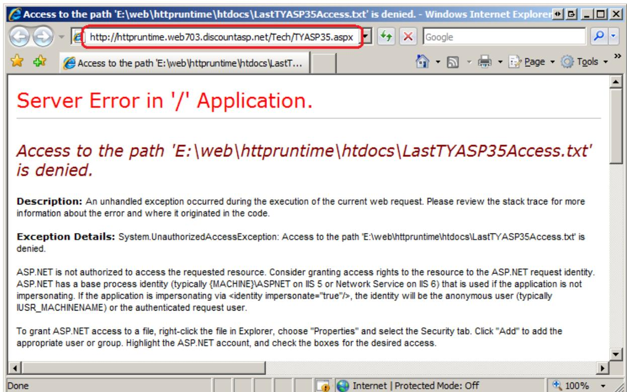
**Figure 2: The Default Machine Account Used by IIS Does Not Have Permissions to Write to the File System**
