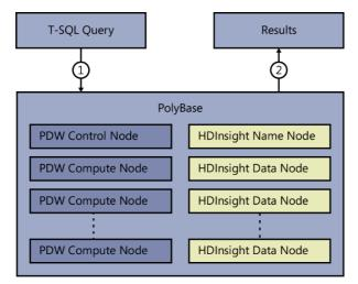
FIGURE 5-5 Schematic diagram of the new Microsoft Analytics Platform System.
