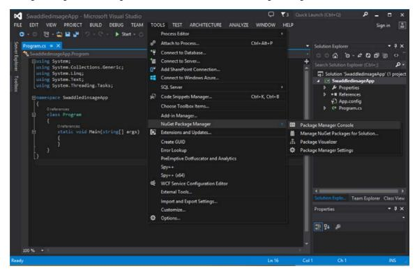
FIGURE 3-4 Launching the Package Manager Console.
