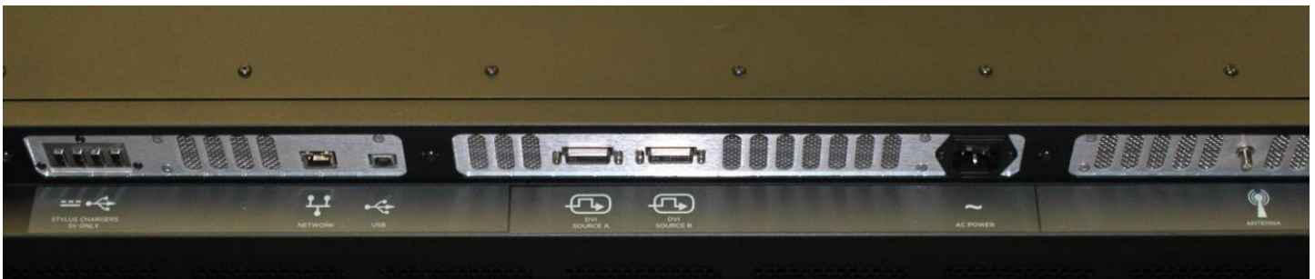
Figure 4. Connection ports from left to right: USB stylus charging, network, USB connectivity, DVI (2), power, and antenna for communicating with stylus
