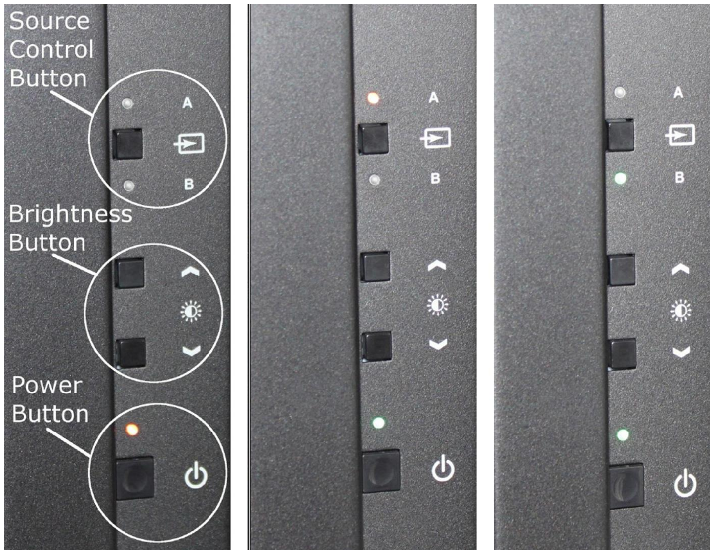
Figure 6. Left: Buttons highlighted with device powered, but no signal as power LED is amber. Center: The device has power and signal, but no signal is coming from the selected source, which has an amber light. Right: The device has power and signal and is getting a signal from the selected source, as both the power and source 'B' LEDs are green
