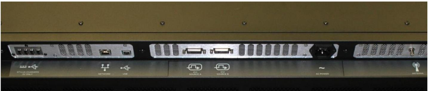
Figure 1. PPI 82" Touch Device connectors
