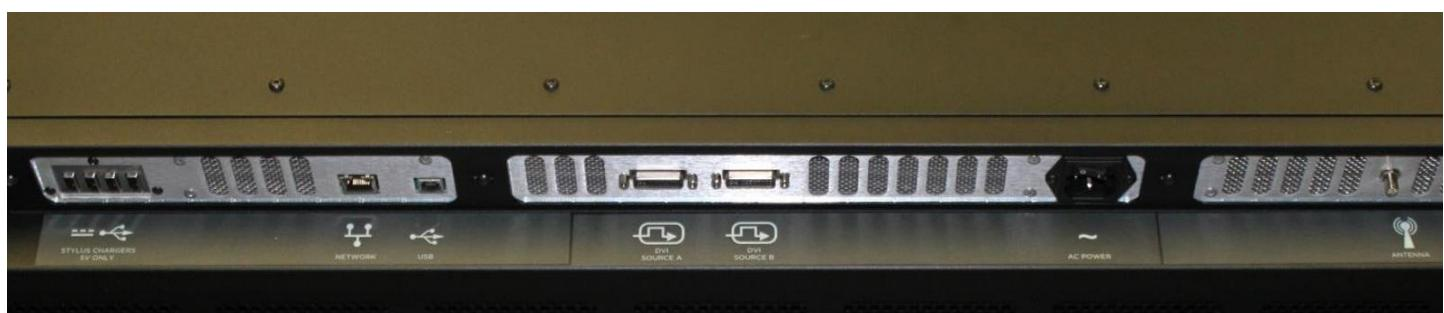
Figure 1. PPI 82" Touch Device connectors
