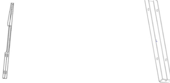
Figure 1. Metal wall mount bracket on the left, metal wall mount locking brackets on the right
