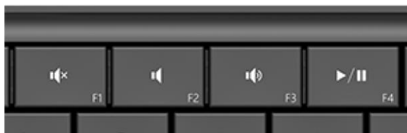
Media keys on Type Cover: Mute, volume down, volume up, and play/pause
