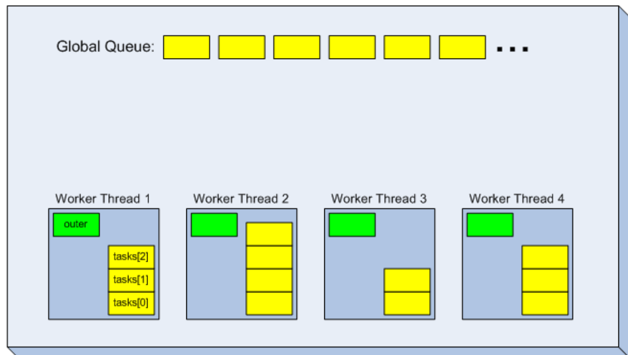
Figure 2: Sample Code Running on Heavily Loaded ThreadPool (green = running, yellow = queued)
