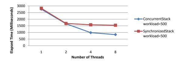
Figure 9: Comparison of scalability for ConcurrentStack(T) and SynchronizedStack(T) in a mixed producer-consumer scenario with a 500 FLOPS workload function.
