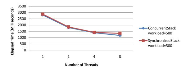
Figure 7: Comparison of scalability for ConcurrentStack(T) and SynchronizedStack(T) in a pure producer-consumer scenario with a 500 FLOPS workload function.
