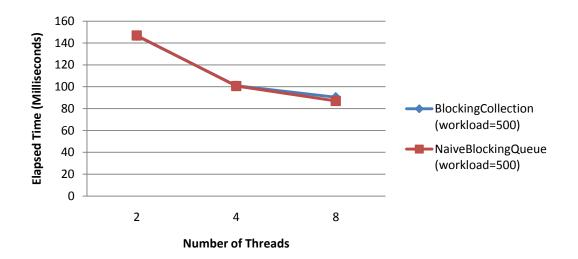
Figure 1: Comparison of scalability for BlockingCollection(T) and NaiveBlockingQueue(T) in the scenario with 1 producer and N-1 consumers and workload of 500FLOPs
