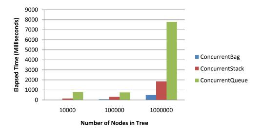
Figure 11: Comparison of ConcurrentBag(T), ConcurrentStack(T), and ConcurrentQueue(T)'s performance in a mixed producer-consumer scenario for various tree-sizes.
