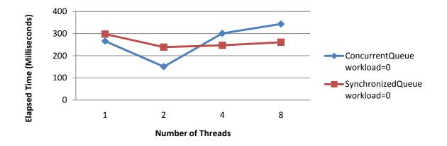
Figure 2: Comparison of scalability for ConcurrentQueue(T) and SynchronizedQueue(T) in a pure producer-consumer scenario with a zerocost workload function.
