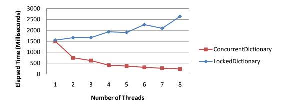
Figure 13: Comparison of scalability for ConcurrentDictionary(TKey,TValue) and SynchronizedStack(TKey,TValue) in a read-heavy producerconsumer scenario.
