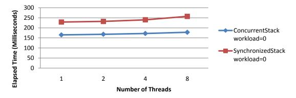
Figure 8: Comparison of scalability for ConcurrentStack(T) and SynchronizedStack(T) in a mixed producer-consumer scenario with a zero-cost workload function.
