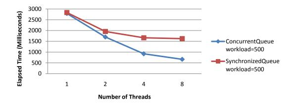
Figure 5: Comparison of scalability for ConcurrentQueue(T) and SynchronizedQueue(T) in a mixed producer-consumer scenario with a 500 FLOPs workload function.
