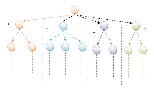
Figure 10: Visualization of graph-traversal using multiple-threads and a ConcurrentBag(T).
