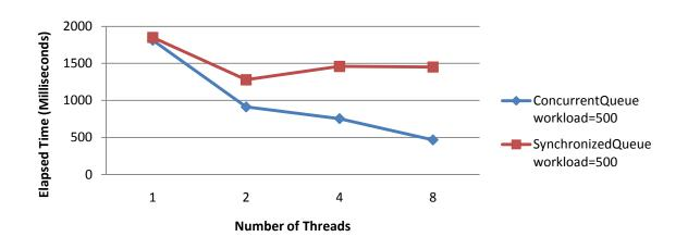
Figure 3: Comparison of scalability for ConcurrentQueue(T) and SynchronizedQueue(T) in a pure producer-consumer scenario with a 500 FLOPS workload function.
