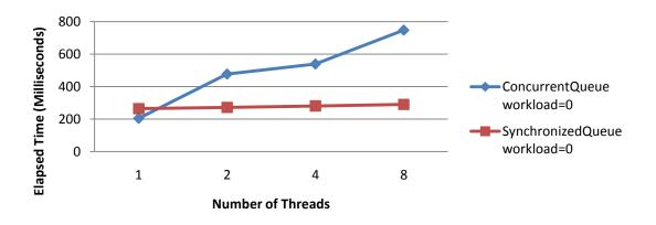
Figure 4: Comparison of scalability for ConcurrentQueue(T) and SynchronizedQueue(T) in a mixed producer-consumer scenario with a zerocost workload function.
