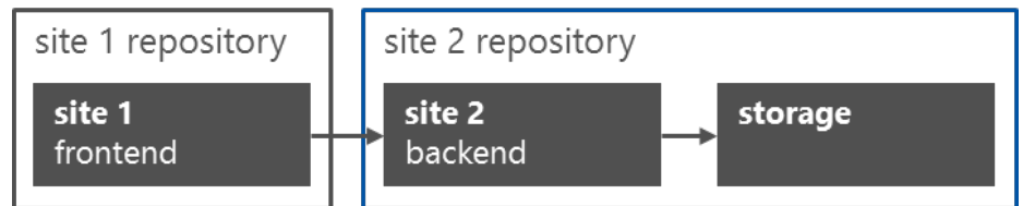
Figure 2: Splitting an application into independent deployable components
