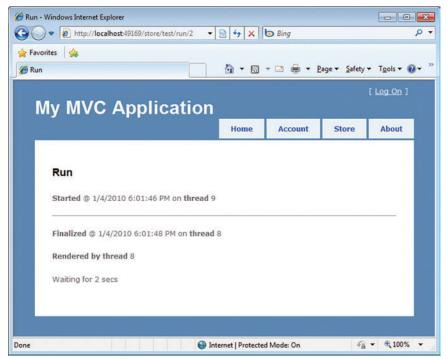
Figure 2 Thread Switching for an Async Action Method Call
