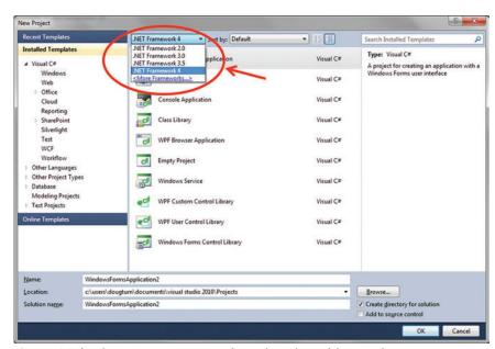
Figure 13 Selecting a Target Framework Version Via Multi-Targeting
