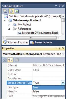
Figure 5 Enabling the Embed Interop Types Feature in Solution Explorer
