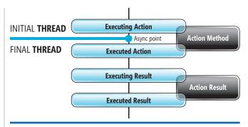
Figure 1 Mechanics of an Async Action Method in ASP.NET MVC
