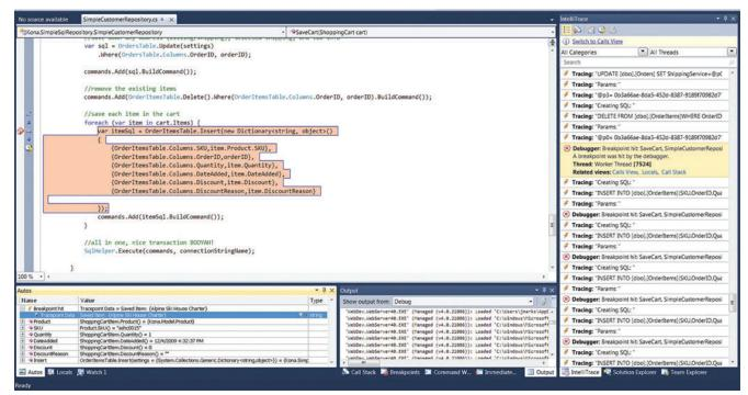
Figure 4 Tracepoints Can Dynamically Add Trace Outputs to Code
