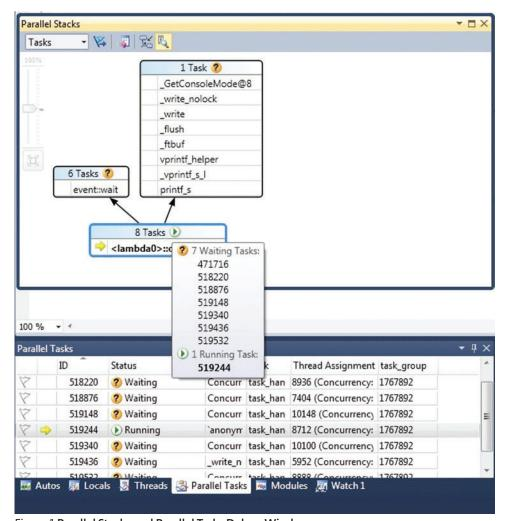
Figure 1 Parallel Stacks and Parallel Tasks Debug Windows
