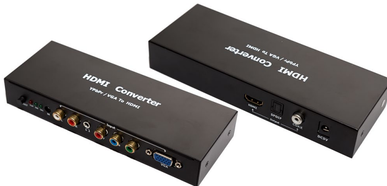
Figure 17-14 Use an HDMI converter for devices that lack HDMI output.
