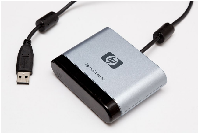
Figure 17-20 Use a USB IR receiver to control your computer with a remote control.
