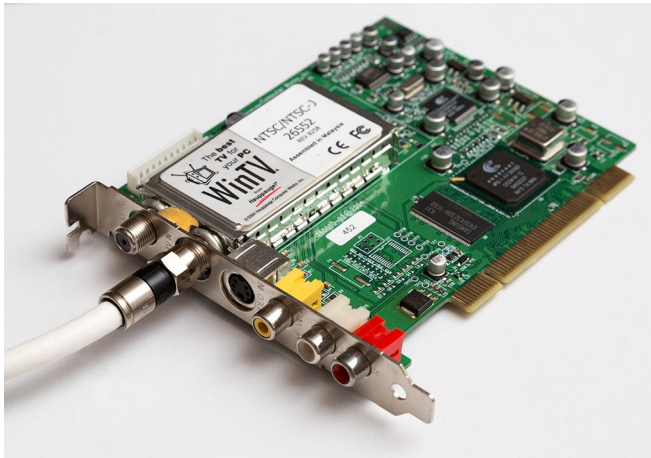
Figure 17-19 Use a tuner card to record TV from analog cable.
