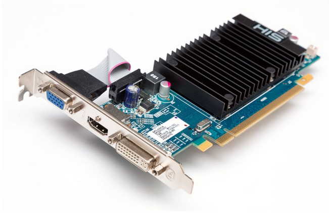
Figure 17-11 To simplify wiring, choose a video card that supports HDMI output.
