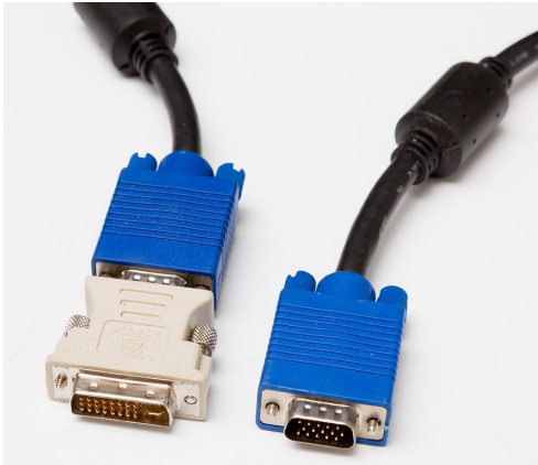
Figure 17-12 Convert between VGA and DVI using an adapter.
