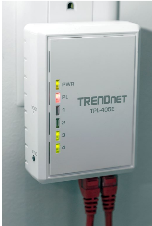
Figure 17-18 Powerline networking can provide the consistent bandwidth you need for streaming HDTV.
