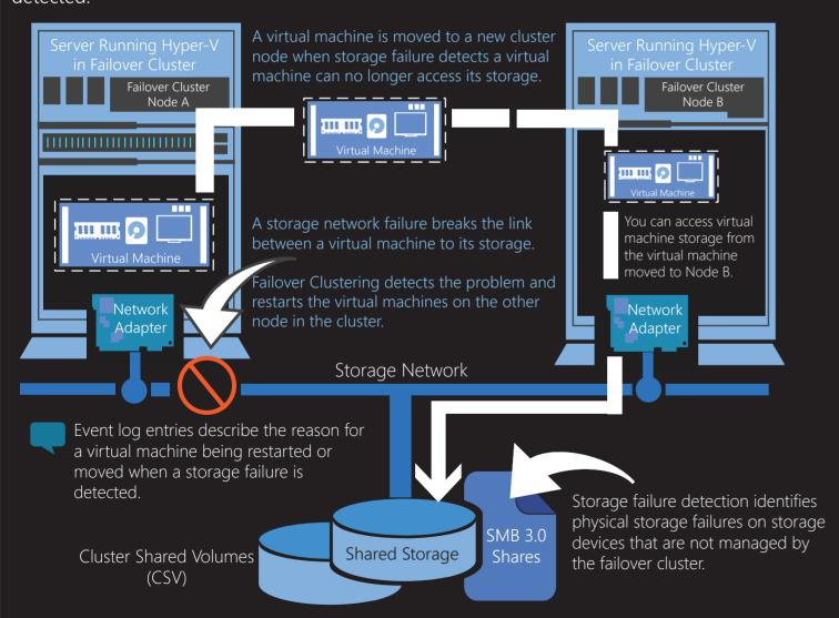
Storage failure detection supports VHD and VHDX file formats, differencing disks, virtual hard disks connected to IDE controllers, virtual hard disks connected to SCSI controllers, virtual machine checkpoints (snapshots), and virtual machines using storage and network resource pools.
