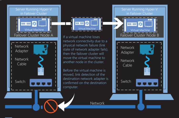
Network failure detection works with any virtual machine. It supports legacy and software-based network adapters, SR-IOV—enabled network adapters, virtual machine checkpoints, storage or network resource pools, and advanced networking features enabled on virtual machines.
