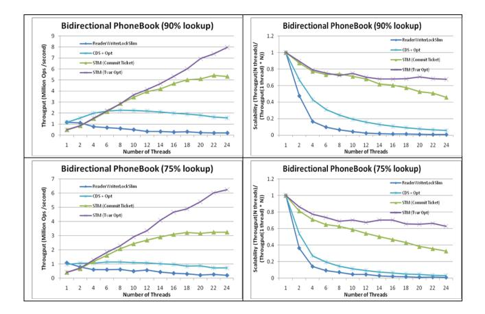
The CDS and optimistic concurrency control based version only achieve best throughput on the readonly case. In all other cases, the STM version performs better than the CDS version as well as the readerwriter lock version significantly. So in other words STM allowed here the reuse of existing code in a very straight forward manner while retaining excellent scalability characteristics.
