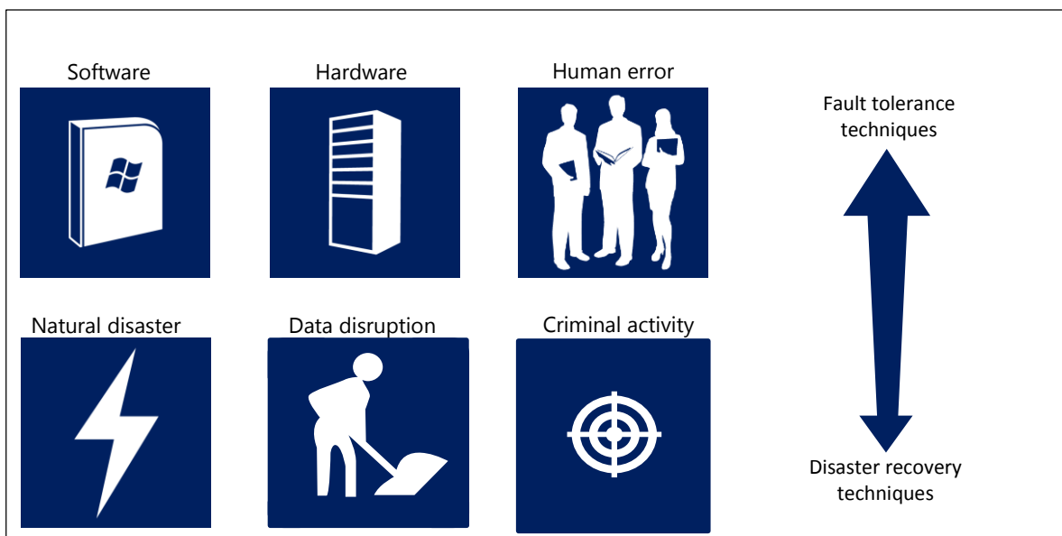
Figure 1. The spectrum of failure ranges from common failures to infrequently occurring failures. Failure is inevitable, so fault tolerance techniques should be incorporated into the service design to reduce the impact when failures occur.
