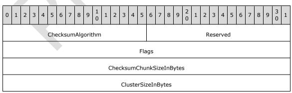
The FSCTL\_GET\_INTEGRITY\_INFORMATION\_BUFFER data element is as follows.
