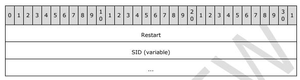
**Restart (4 bytes):** A 32-bit unsigned integer value that indicates to restart the search. This value MUST be 0x00000001 on the first call so that the search starts from the beginning of the directory on which the operation is requested. For subsequent calls, this member SHOULD be zero so that the search resumes at the point where it stopped.
