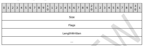
The FSCTL OFFLOAD WRITE OUTPUT data element is as follows.
