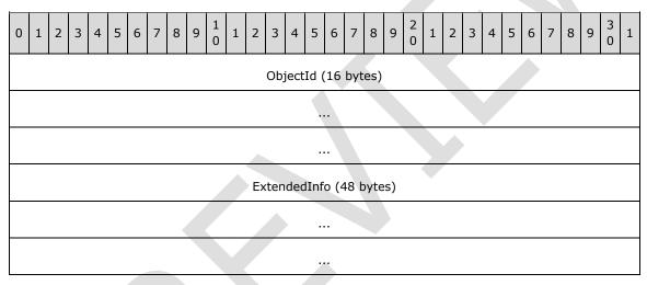
**ObjectId (16 bytes):** A 16-byte GUID that identifies the file system volume on the disk. This value is not required to be unique on the system.
