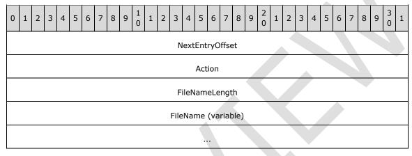
NextEntryOffset (4 bytes): The offset, in bytes, from the beginning of this structure to the subsequent FILE\_NOTIFY\_INFORMATION structure. If there are no subsequent structures, the NextEntryOffset field MUST be 0. NextEntryOffset MUST always be an integral multiple of 4. The FileName array MUST be padded to the next 4-byte boundary counted from the beginning of the structure.
