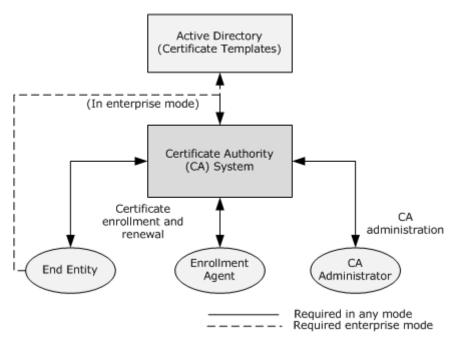
Figure 3: CA System external interfaces
