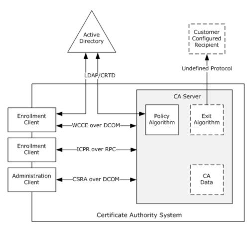
Figure 8: The CA System as an enterprise CA
