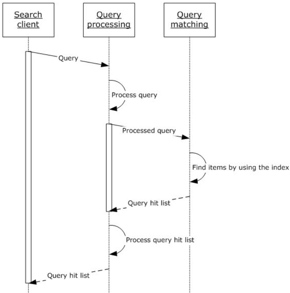
**Figure 14: Sequence diagram for performing a query**
