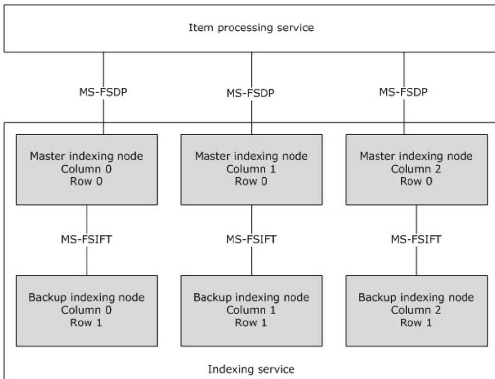
**Figure 10: Indexing service configured across three index columns**
