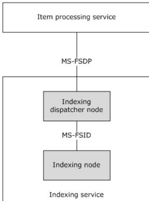
**Figure 9: Relationship between components of the indexing service**
