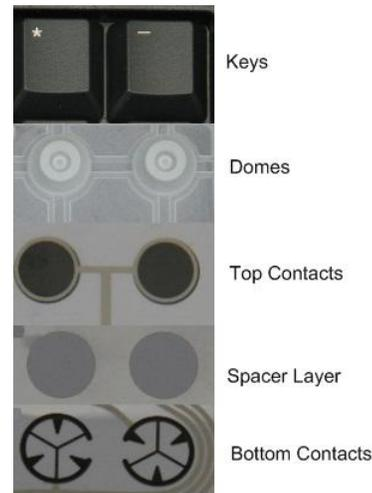
Figure 2: Pressure sensitive keyboard design. When a key is pressed, the top contact deforms through the spacer, making more or less contact with the carbon traces on the bottom layer. This yields a pressure dependent resistance.
