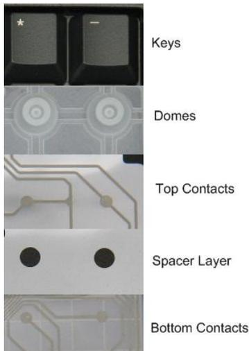
Figure 1: Flexible membrane/rubber dome keyboard construction. Keys press on rubber domes that provide the appropriate tactile sensation. In turn, the domes press on a stack of three membranes. When a key is pressed, the top sheet deforms through a hole in the spacer layer, making electrical contact with the bottom sheet.
